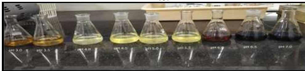
Fig. 1 (a) Variation in colour removal efficiency of the coagulants at different (b) intensity of colour observed in leachate treated with \text{FeCl}_3 at various pH. (c) Intensity of colour observed in leachate treated with \text{FeSO}_4 at various pH. (d) Intensity of colour observed in leachate treated with alum at various pH
