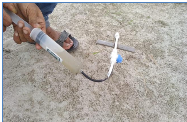
Fig. 5 Soil sediment water pore sampler developed for SGD sample collection
