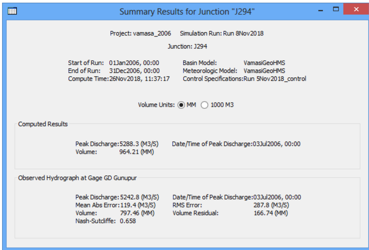
Figure 2. Model calibration at Gunupur GD of Vamasadhara river basin
