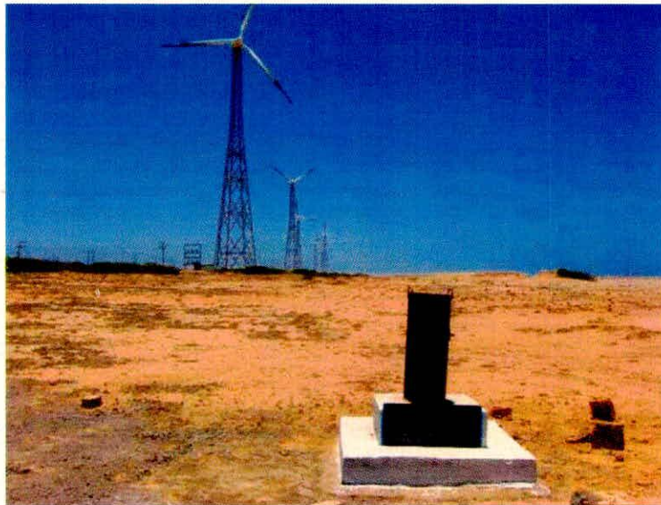
Piezometer installed near sea coast in Porbandar (Gujarat) to monitor cyclic water table fluctuations induced by tidal fluctuations.
