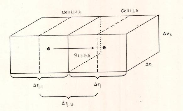
Figure 4.—Flow into cell i,j,k from cell i,j-l,k.
