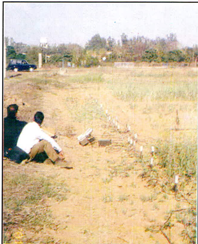
Figure – 1 Setup of resistivity electrodes
