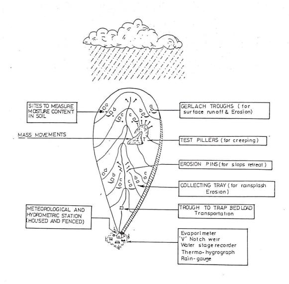
Fig. 2: Watershed Instrumentation
