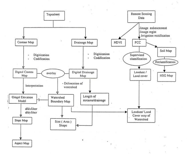
Fig. 1 Steps involved to determine various watershed characteristics by using GIS and Remote Sensing
