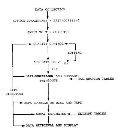
FIGURE 1 - FLOW CHART SHOWING THE GENERAL DATA PROCESSING FRAME WORK
