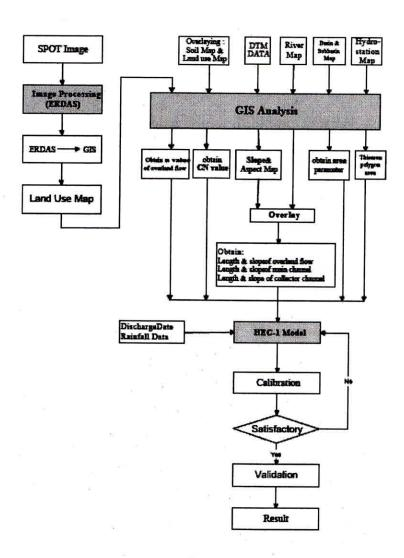
Fig. 1: Flow Chart showing RS & GIS data use in HEC-1 Model
