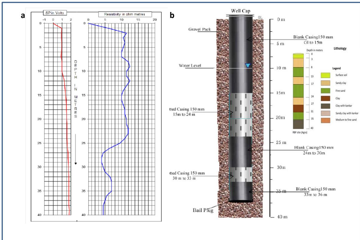
**Fig. 9.** (a) Design and lithology of the exploratory bore well showing tapping zone, (b) SP and resistivity profiles of bore well at Agra site
