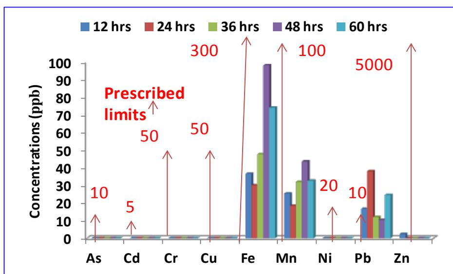
Fig. 11. Trace metal concentration in bore well water at Agra site
