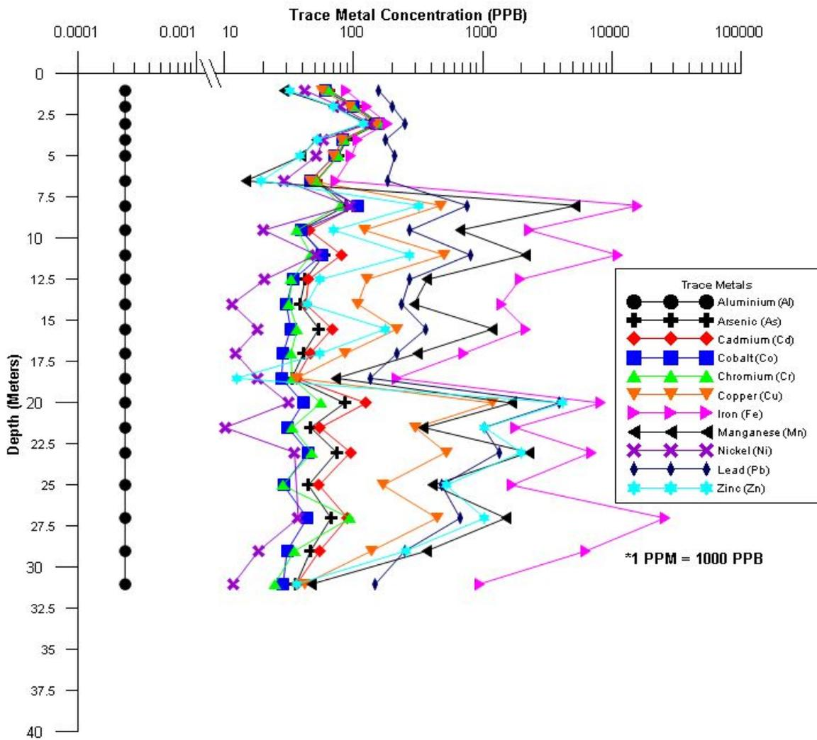
Fig. 10. Trace metal concentration in soil core samples at Agra site
