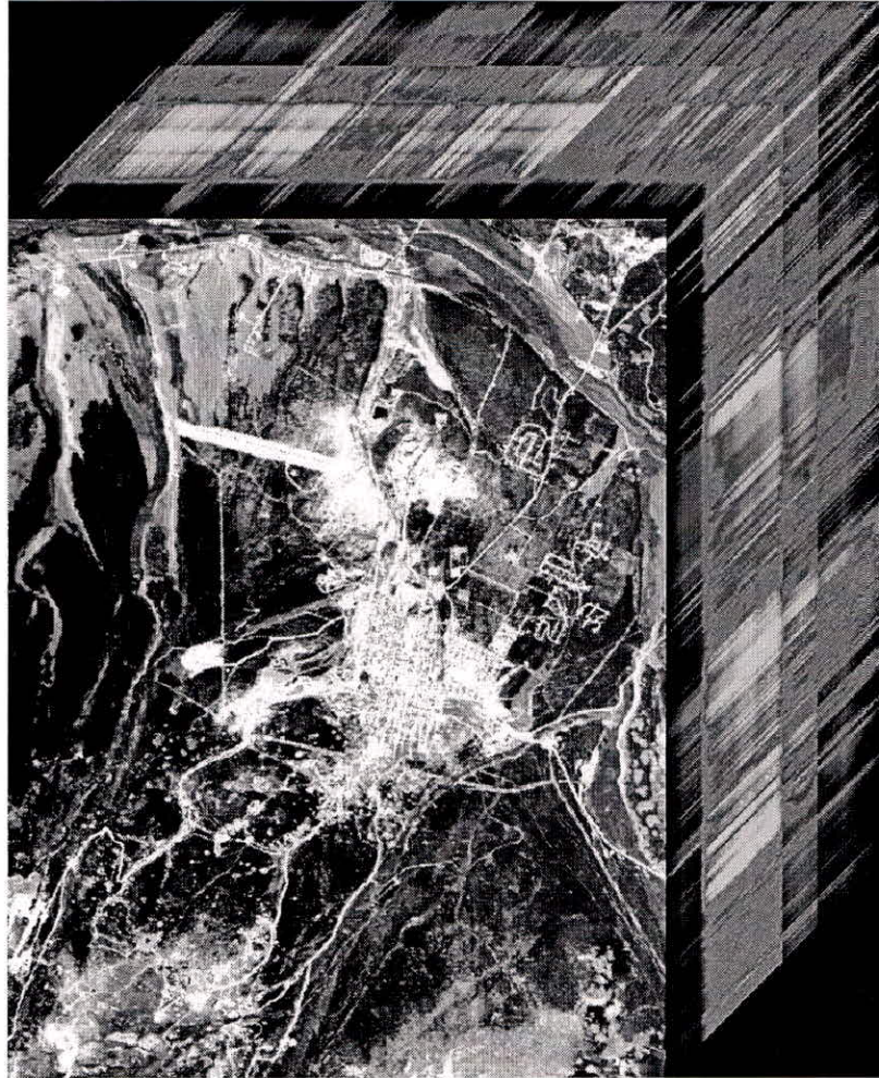
Figure 2. Hyperspectral images are sometimes referred to as “image cubes” because they have a large spectral dimension as well as the two spatial dimensions. This cube shows an AVIRIS hyperspectral image of the Leadville mining district in Colorado, with the spectral dimension shown as the top and right faces of the cube. The front of the cube is a true color composite, with areas containing secondary minerals from acid mine drainage highlighted in red, orange and yellow.
