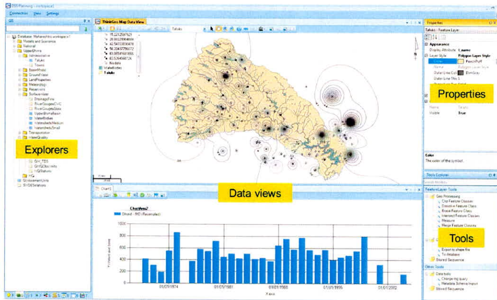
Figure 2-1. DSS (P) Planning Interface including the GIS and Time Series Explorers as well as directories of all the GIS coverages and the properties and tools explorers for editing and operating on the maps and charts.
