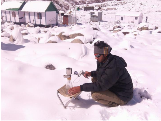
Fig. 3.9 On-site water sample filtration for suspended sediment
