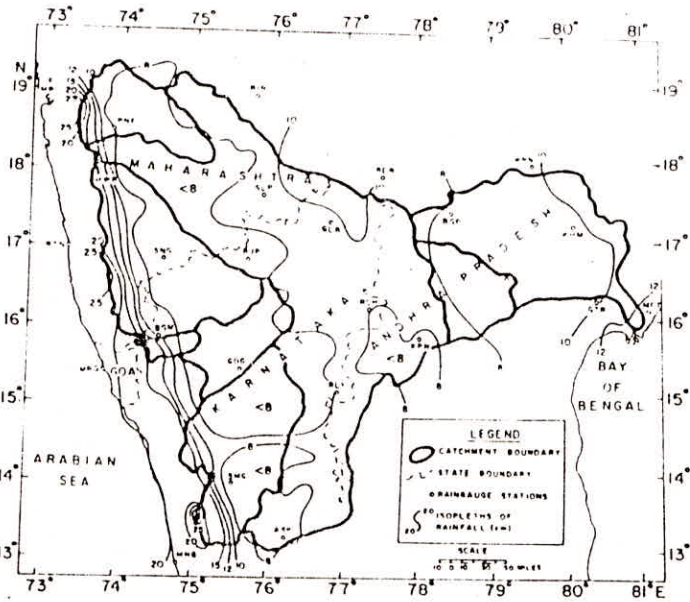
Fig. 1 : Generalized chart of 2-Year one-day maximum rainfall (in cm) of the Krishna Catchment.
