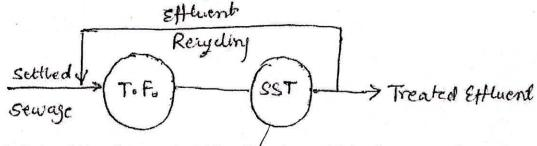
A distinguishing feature of trickling filter from ASP is, that a part of treated effluent from secondary settling tank is recycled back into the filter whereas, a part of secondary sludge is recycled back in aeration tank in ASP.
