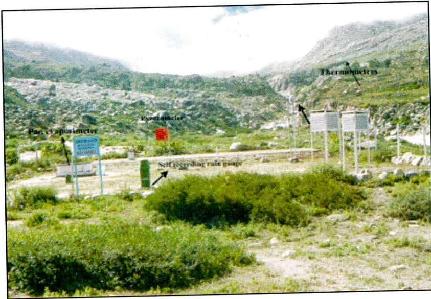
Plate 8 : Meteorological Instruments: Thermometers, Pan –evaporimeter, Pyrenometer, Self recording rain gauge.
