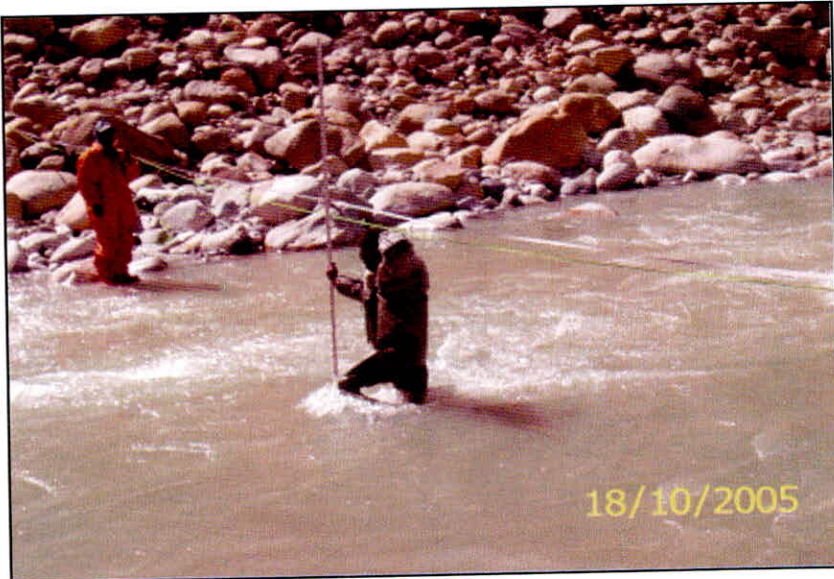
Plate11: Cross section observations from the Gauging well at Bhagirathi River near Bhojwasa.
