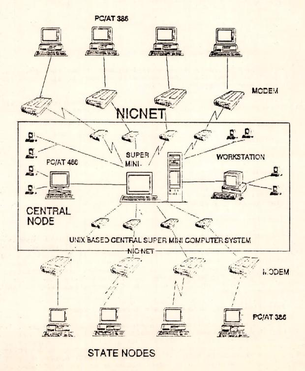
FIG.1-DIAGRAM SHOWING LINKAGE OF CENTRAL, STATE AND REGIONAL NODES
