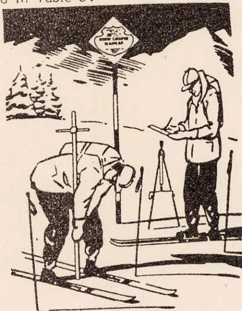
Fig.23 Snow sampling in the field by the use of snow samplers
