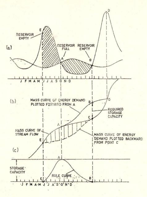
FIG.2 THE STREAMAFLOWS OF A RIVER AND THE WATER REQUIREMENTS
