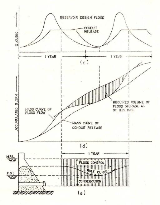
FIG.3 ANNUAL PLANS OF OPERATION OF A MULTIPURPOSE RESERVOIR
