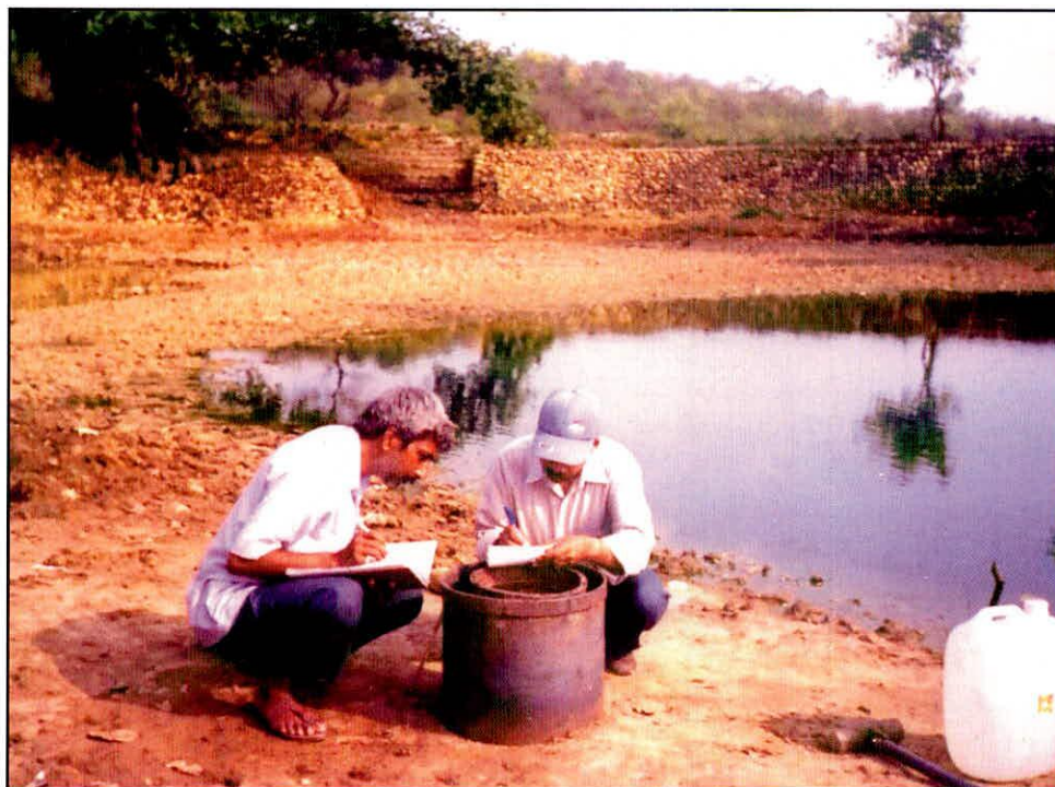
Fig. - 5.2: A view of infiltration test being carried out in a pond
