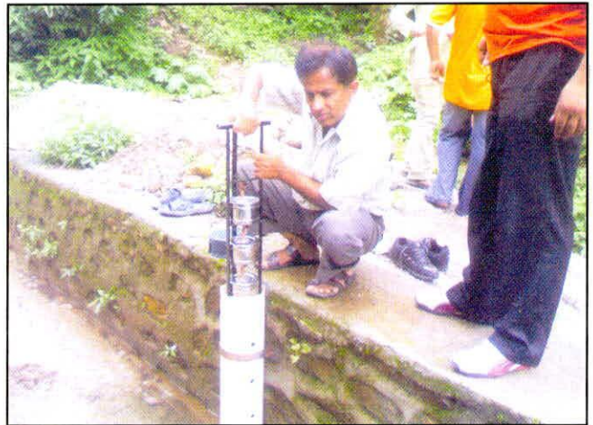
Low cost storm water sampler and its installation at Arnigarh and Bansigarh watersheds
