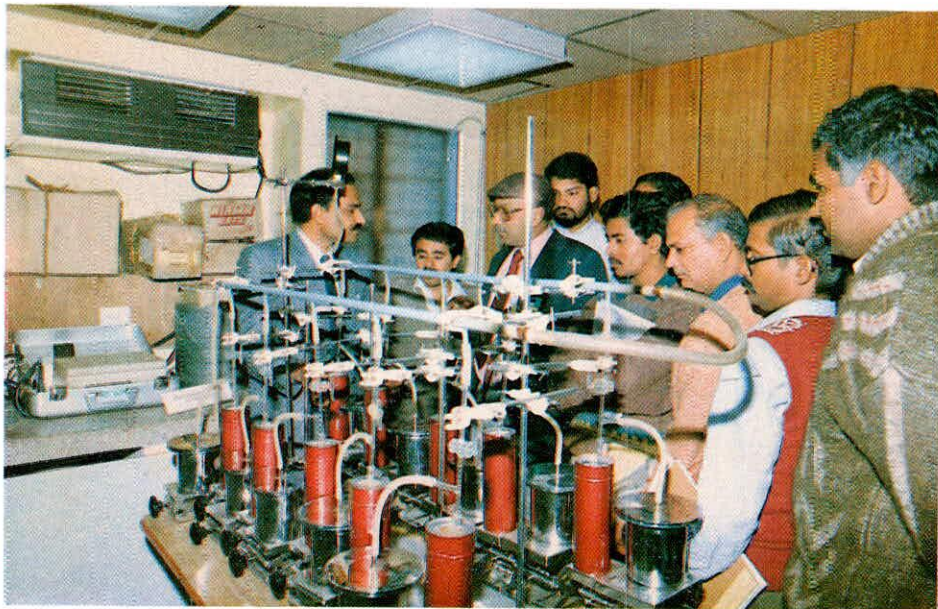
Visiting Trainee Officers being shown Soil Moisture Extraction Unit in Nuclear Hydrology Laboratory
