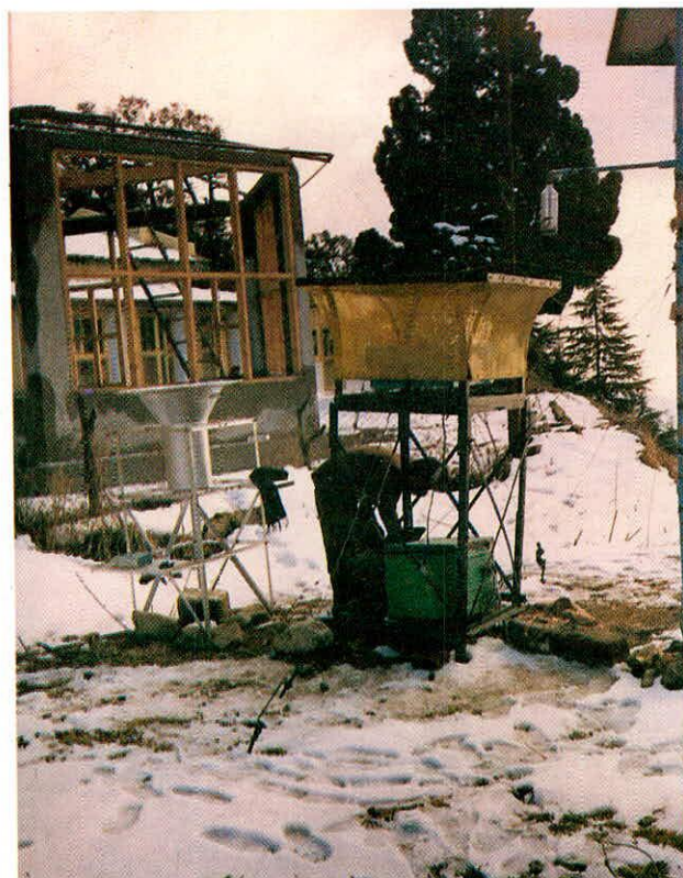
Field Testing of Weighing Type Snow Gauge at Dhanaulti, UP
