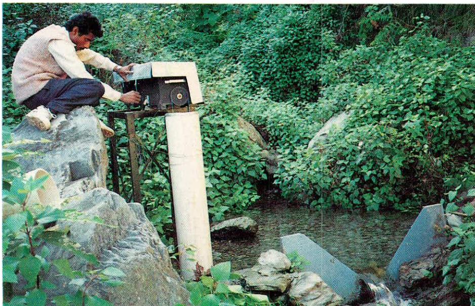
Installation of Automatic Water Level Recorder at Discharge Measuring Site in Danda Watershed under DST Sponsored Project.
