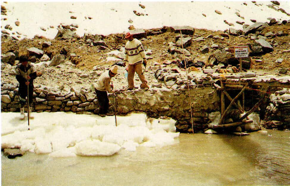
NIH Expedition Team to Dokriani Glacier Removing Snow from the Stream for Accurate Discharge Measurement.
