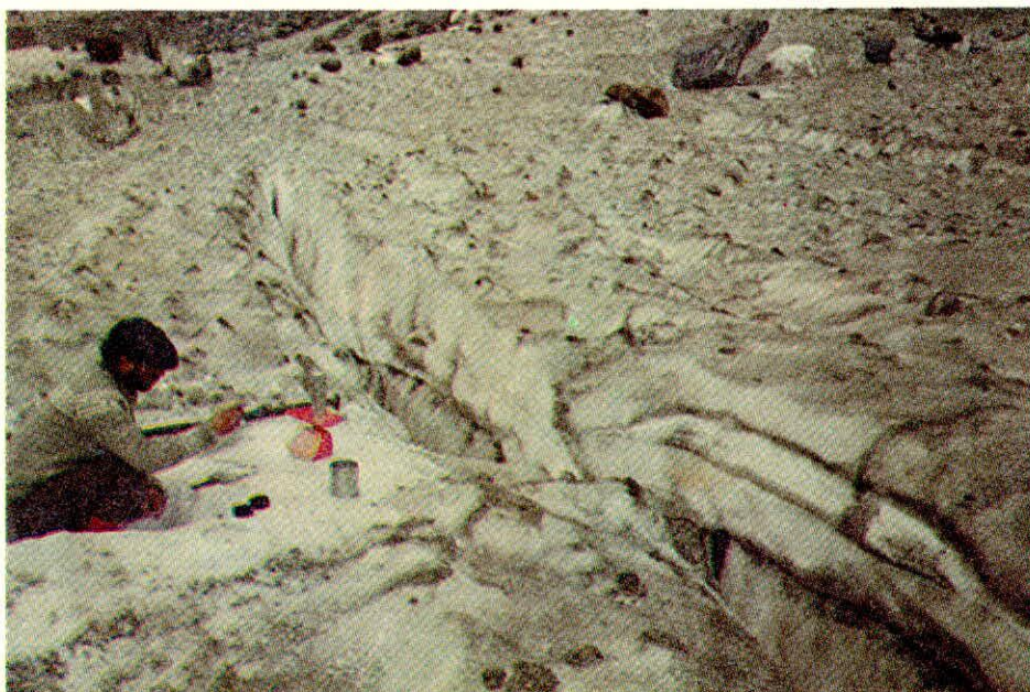
Fig.4 - Snowpack stratigraphic study by digging a pit
