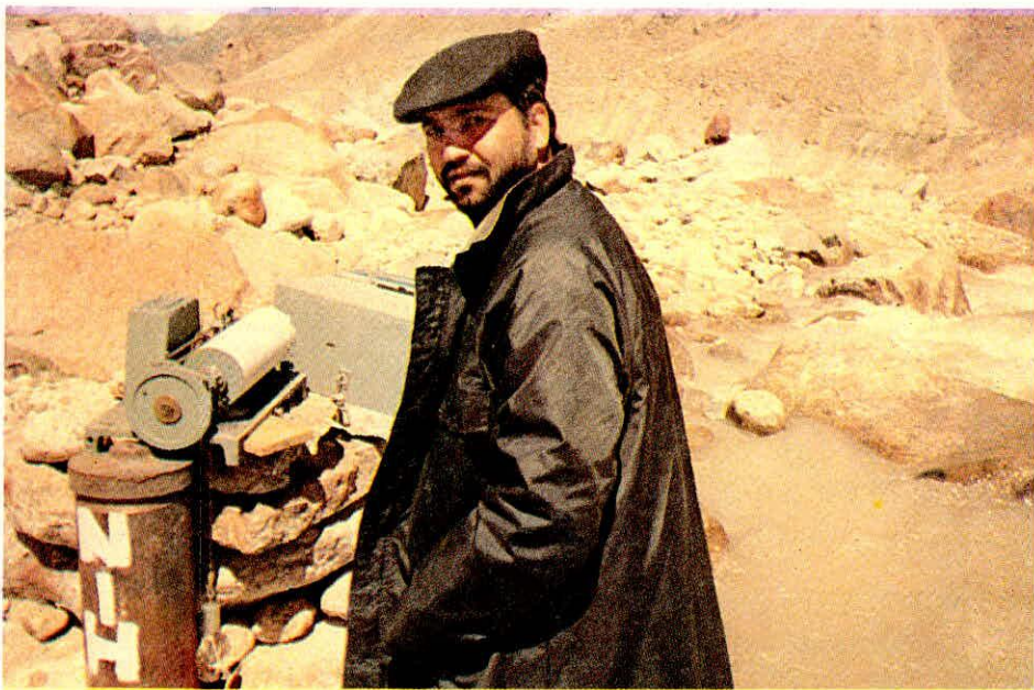
Fig.12 - Water level recorder installed at the gauging site
