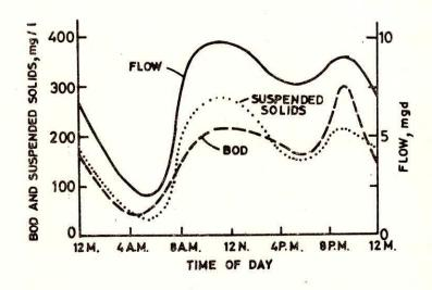
FIG.1-TYPICAL HOURLY VARIATION IN FLOW AND STRENGTH OF DOMESTIC SEWAGE (SOURCE METCALF & EDDY, INC. 1972)
