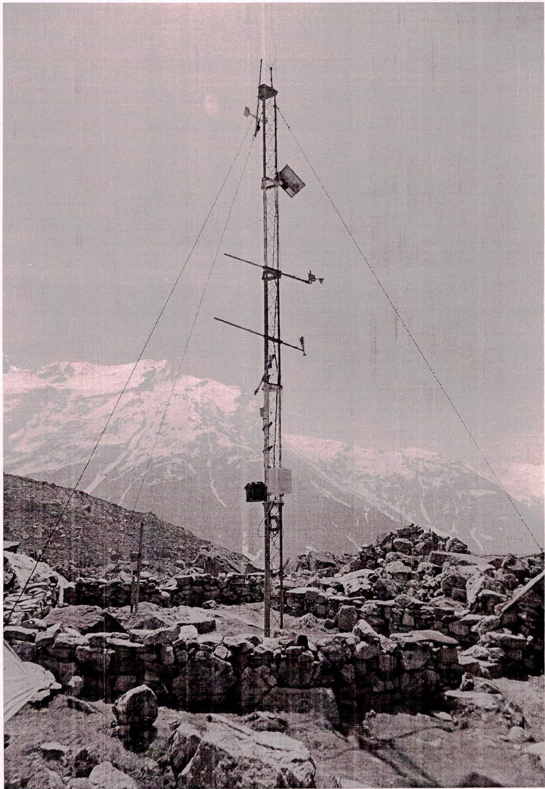
Fig. 4.1: Complete setup of Automatic Weather Station installed at Base camp site (3820 m a.s.l.) of the Chorabari Glacier, Garhwal Himalaya (Source: Kesarwani, 2015).
