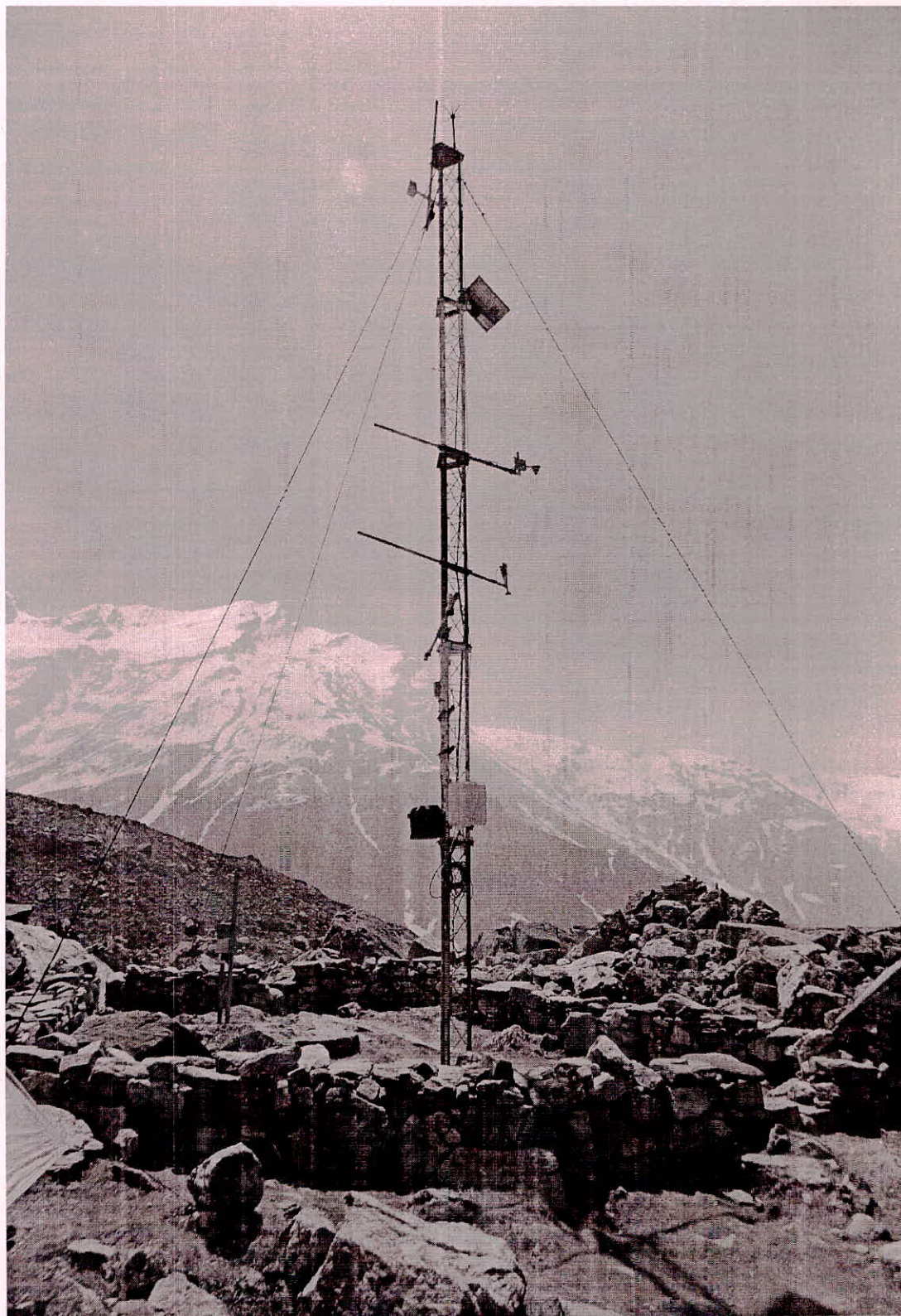
Fig. 4.1: Complete setup of Automatic Weather Station installed at Base camp site (3820 m a.s.l.) of the Chorabari Glacier, Garhwal Himalaya (Source: Kesarwani, 2015).
