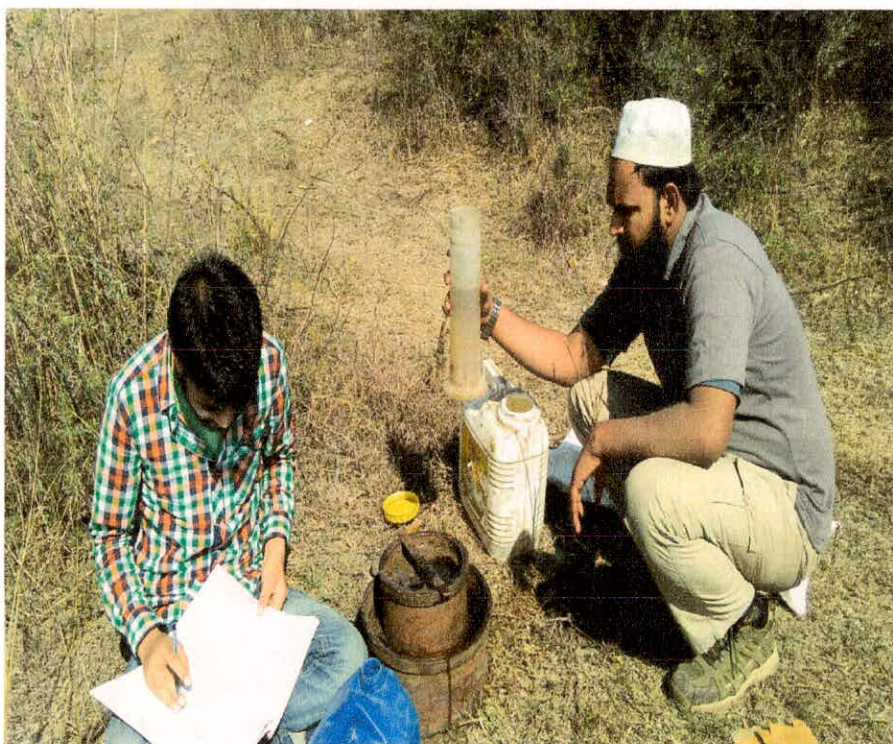
Figure14: Field Measurement of Infiltration Using Double Ring Infiltrometer.
