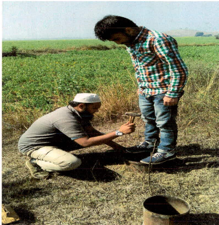
Figure 13: Process of Double Ring Infiltrometer
