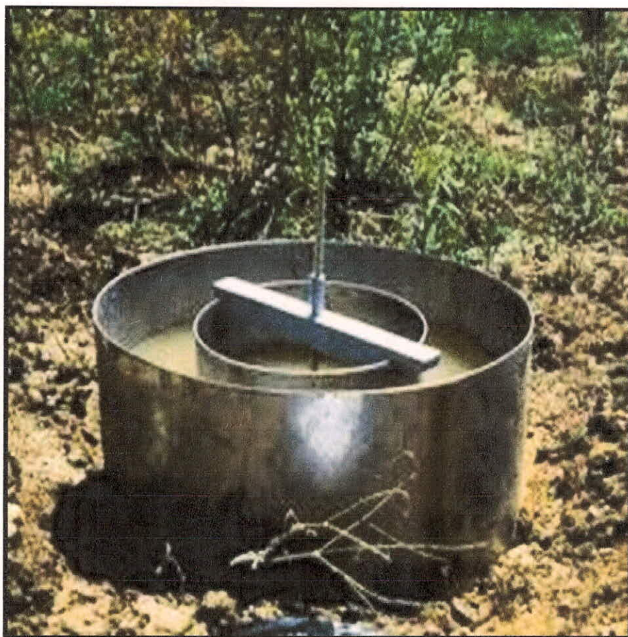
Figure 10 : Field Set Up of Double Ring Infiltrometer
