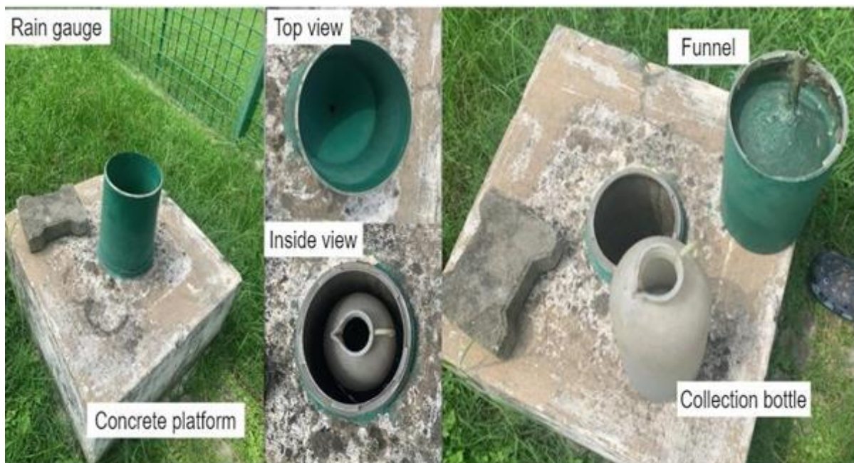
Figure A10: Rain gauge setup for collecting rainwater for isotope analysis.
