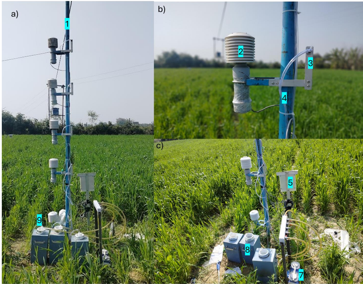
Figure A4: Setup for collection of water vapour. 1) Air Intake structure; 2) Temperature and relative humidity (T and RH) sensor with thermal shield; 3) Sampling port; 4) Teflon tube for sampling air moisture; 5) Data logger for T and RH sensors; 6) Manifold; 7) Vacuum pump; 8) Wooden box for holding Dewar flask; and 9) Cold trap.
