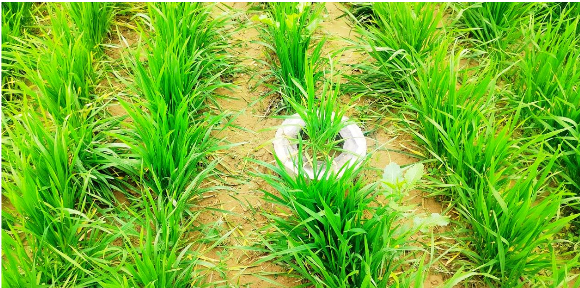
Figure A2: Mini-lysimeter installed in a wheat field at Bithoor. The lysimeter setup is used for continuous monitoring of evapotranspiration (ET) by measuring real-time weight changes in the soil-plant system. The setup includes a high-precision load cell, data logging system, and a protective enclosure.
