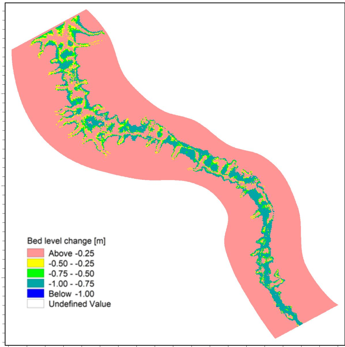
**Figure 5.66: Absolute maximum degradation (erosion) predicted over five years of monsoon.**
