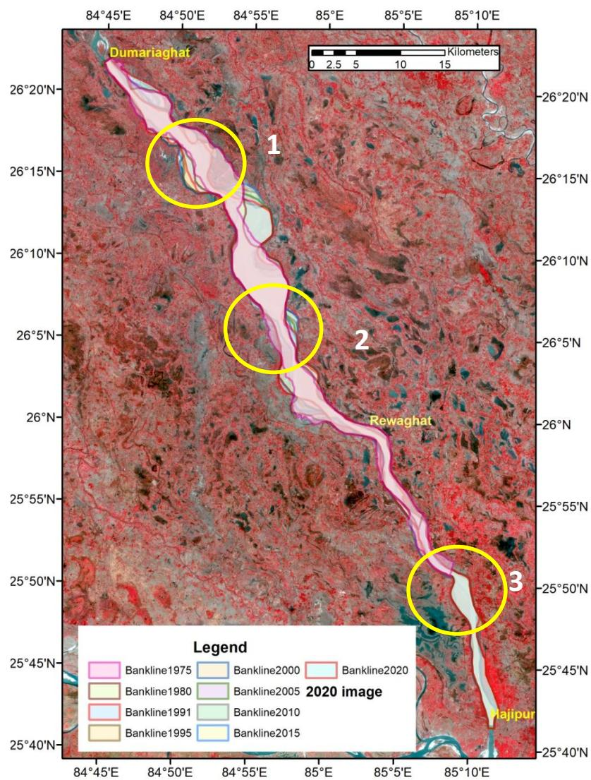
**Figure 5.2: Overlay of the river bank line during 1975 to 2020 extracted from temporal images.**
