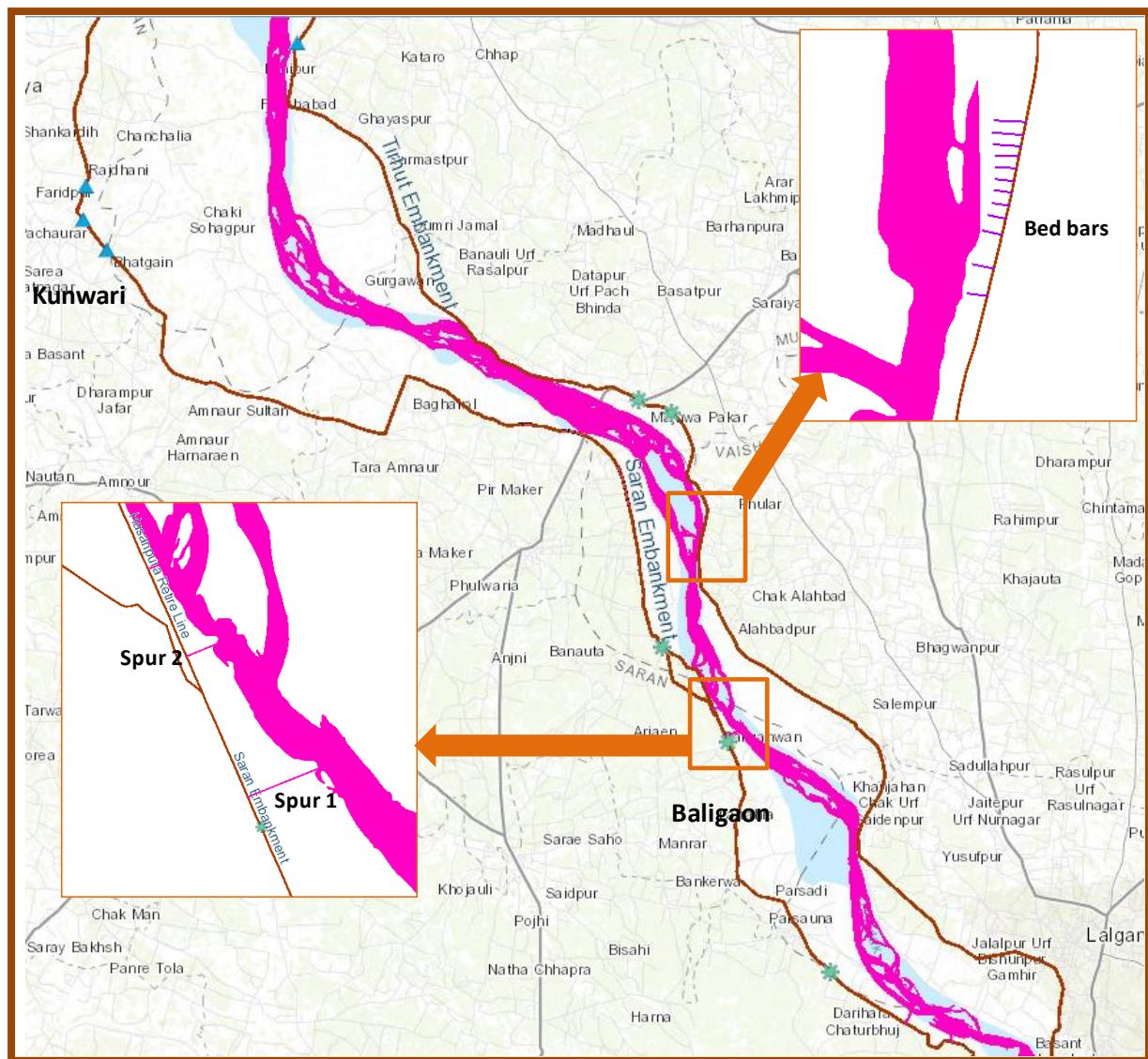
**Figure 2.3: location of anti-erosion structures in the study reach.**
