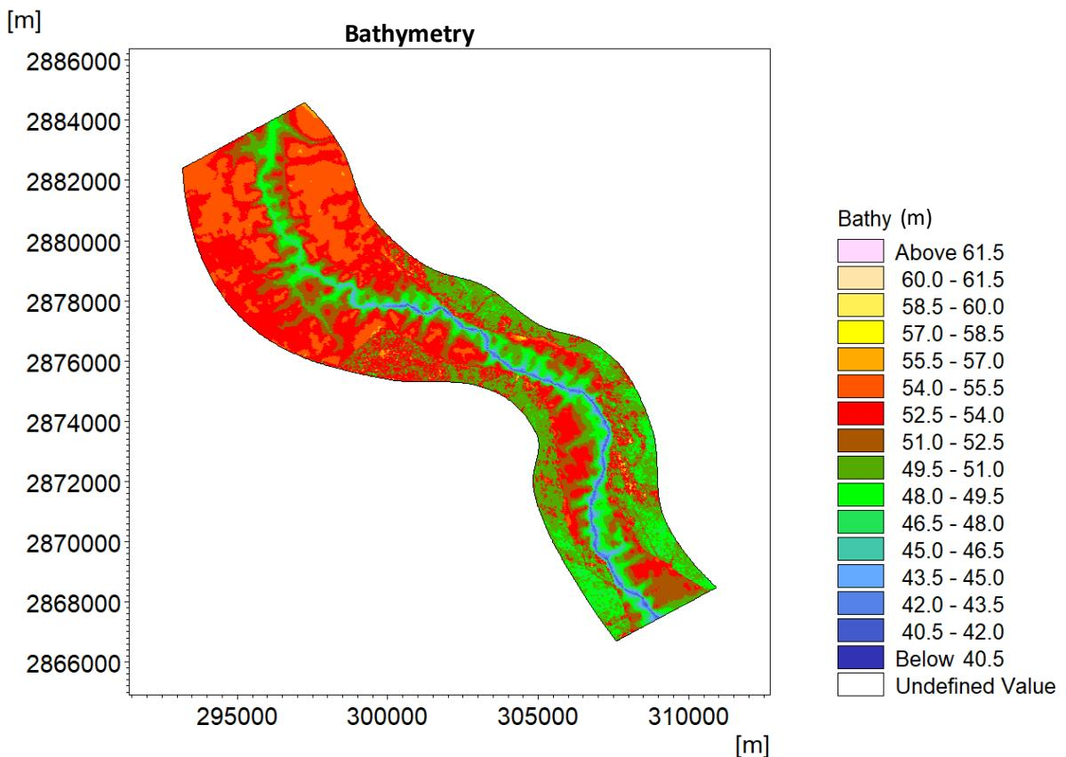
**Figure 5.34: The bathymetry of the Gandak river for curvilinear grid.**
