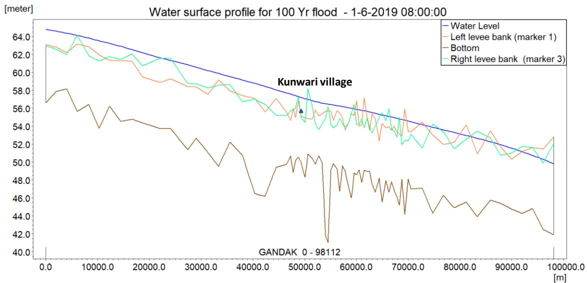
**Figure 5.38: Water Surface profile in Gandak river for 100- Yr flood.**
