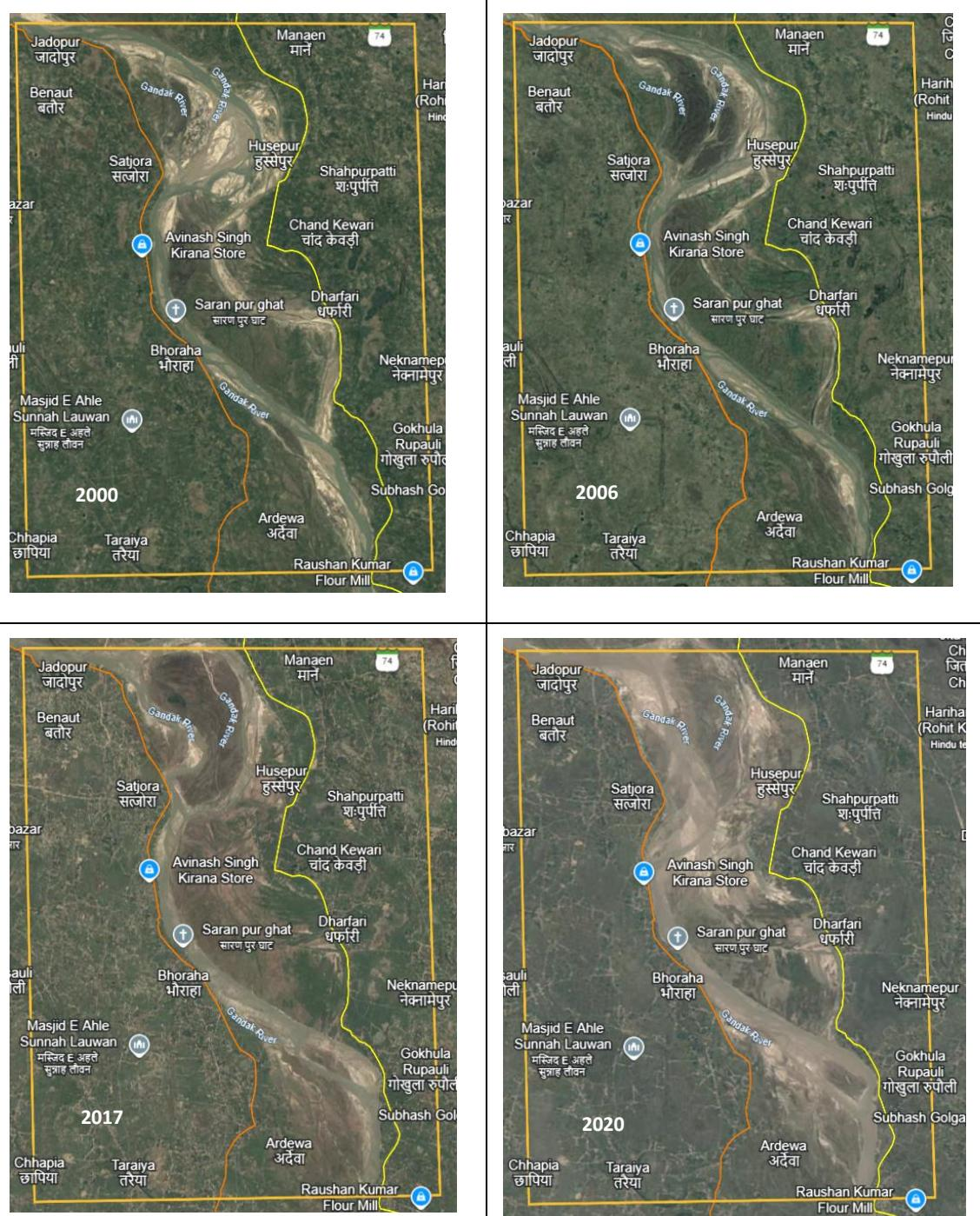
**Figure 5.8: River is shifting between Village Jadopur and Gokhula Rupali in between the embankment since 2000.**
