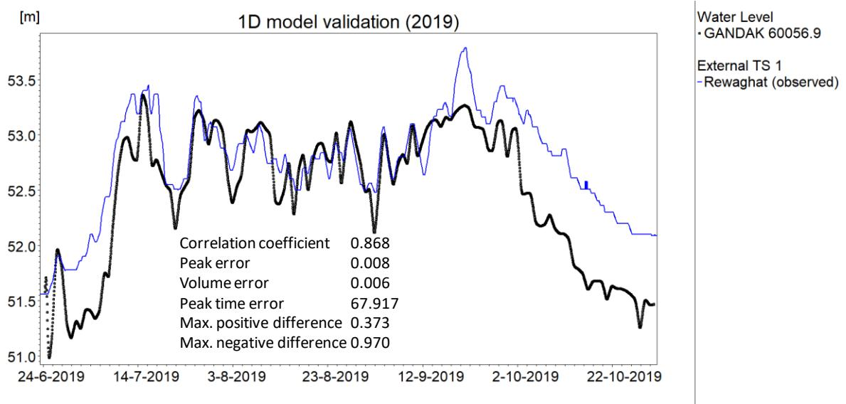
**Figure 5.20: Validation of 1D flow model for 2019 flow data.**
