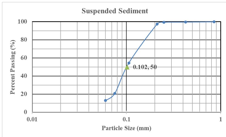
**Figure 3.12: Grain size distribution chart for suspended sediment.**
