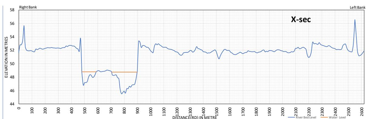
**Figure 3.6: River cross section at the Baligaon site**
