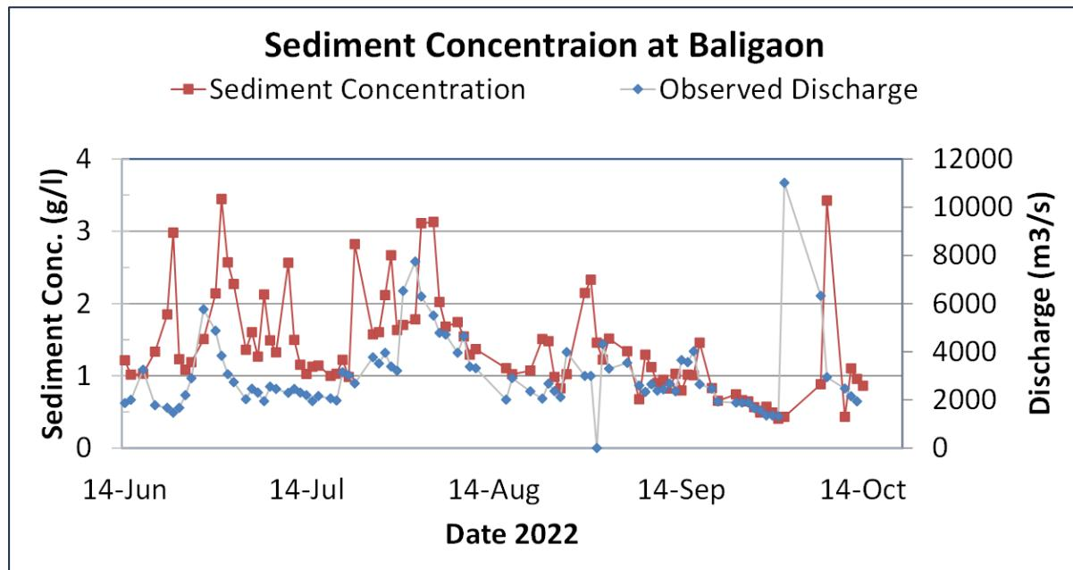
**Figure 3.11: Hydrological data collected by NIH at Baligaon**
