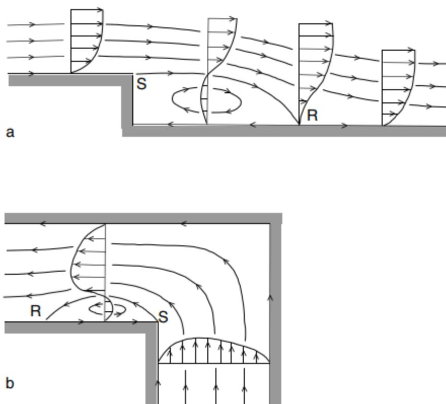
**Figure 4.2: Examples of flow separation (S: separation point; R: reattachment point), illustrated by time-averaged streamline patterns at (a) a downward transverse step and (b) a sharp bend in an open channel.**
