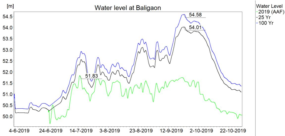
**Figure 5.23: Maximum flood levels computed at Baligaon village for various flood estimates.**
