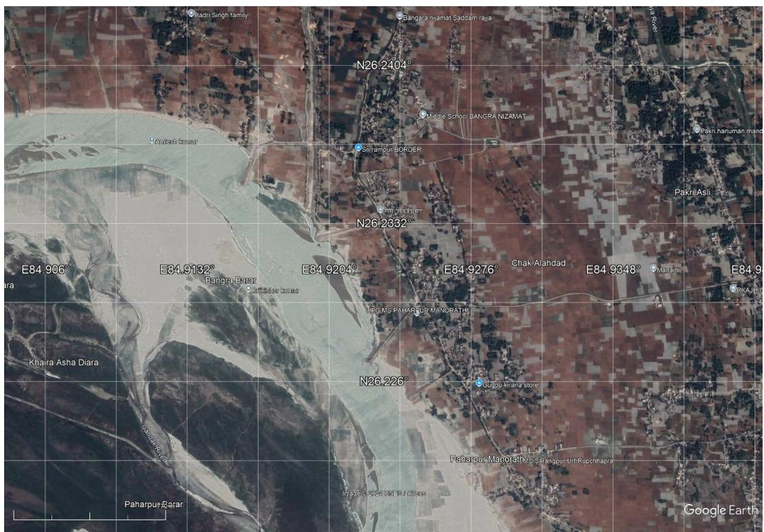
**Figure 5.5: The shifting is controlled due to anti-erosion works and construction of embankments at village Munja and Chak Alahdad appearing in 2013 images in Google Earth Images.**
