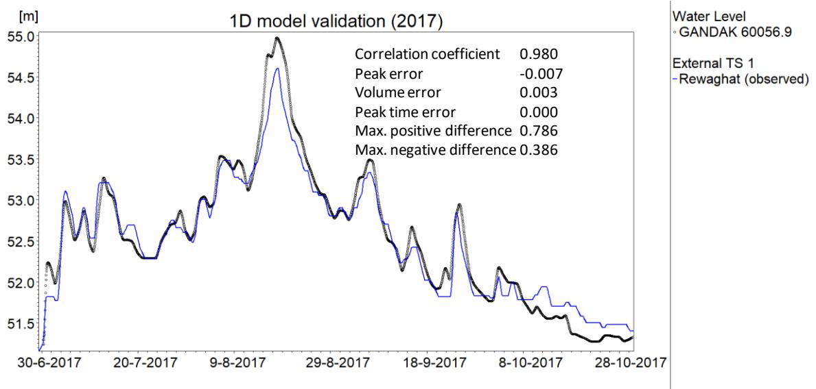
**Figure 5.18: Validation of 1D flow model for 2017 flow data.**
