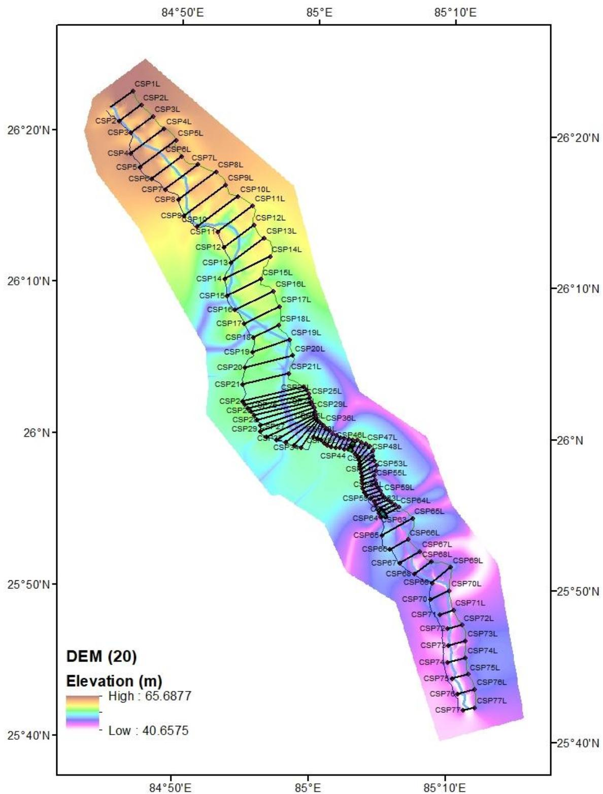
**Figure 3.15: The surveyed cross sections and the DEM of the river reach.**
