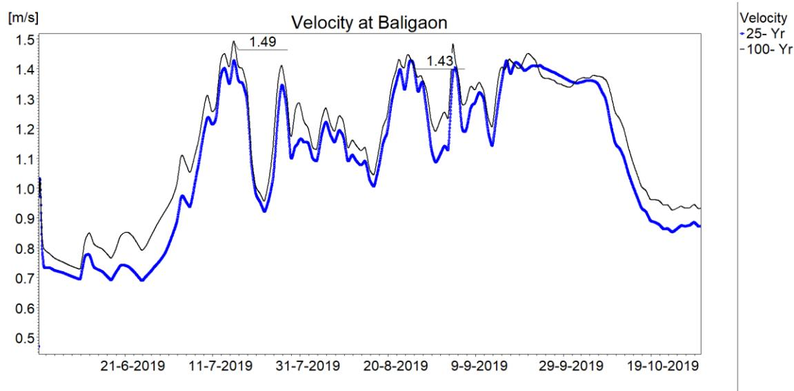
**Figure 5.25: Maximum flow velocities computed at Baligaon village for various flood estimates.**
