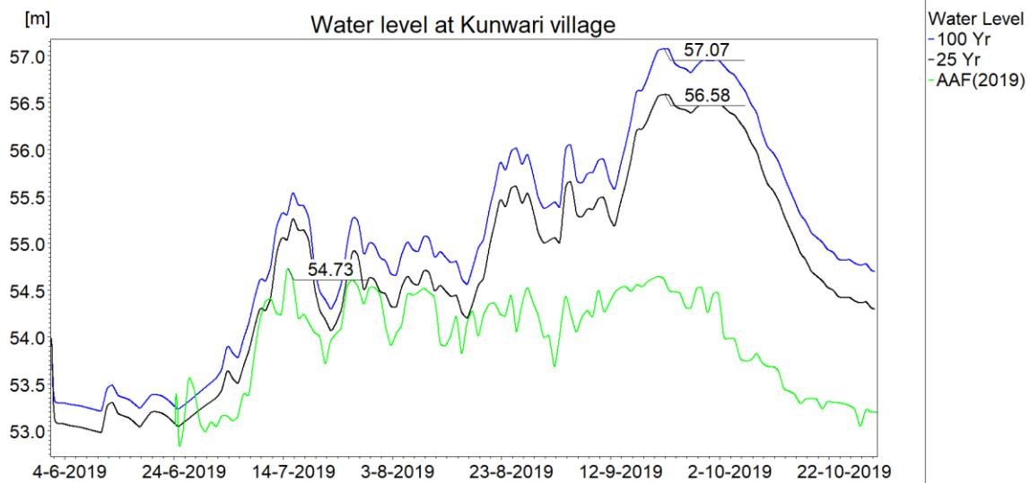
**Figure 5.22: Maximum flood levels computed at Kunwari village for various flood estimates.**
