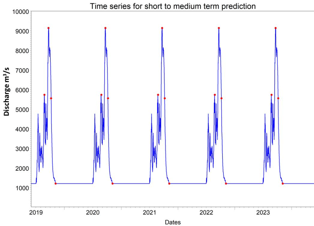
**Figure 5.60: Flood hydrograph for short to medium term prediction.**
