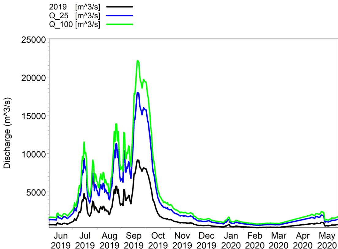
**Figure 5.14: Observed flood hydrograph for 2019-2020 and the scaled hydrograph for 25- and 100- year return period at Dumariaghat GD site.**
