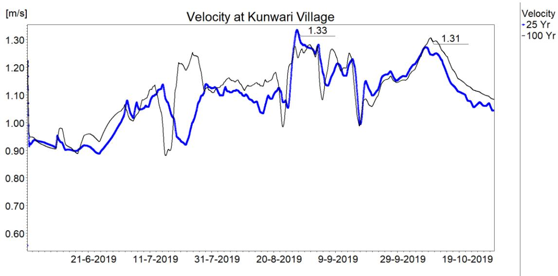
**Figure 5.24: Maximum flow velocities computed at Kunwari village for various flood estimates.**
