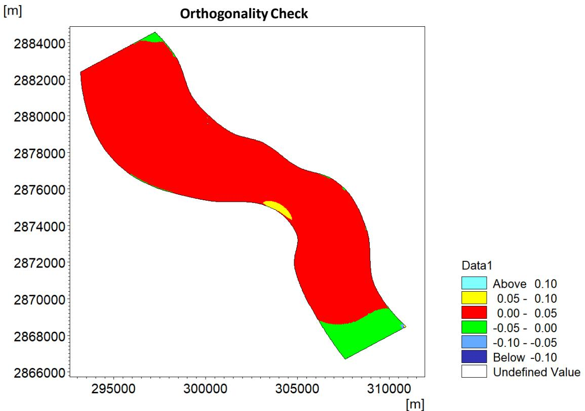
**Figure 5.33: Orthogonality for the curvilinear grid.**
