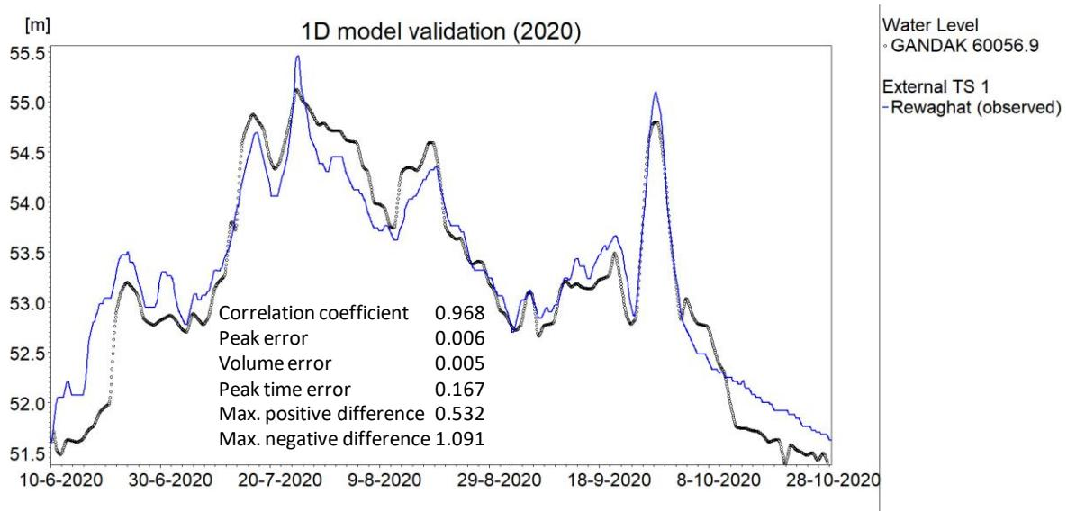
**Figure 5.21: Validation of 1D flow model for 2020 flow data.**
