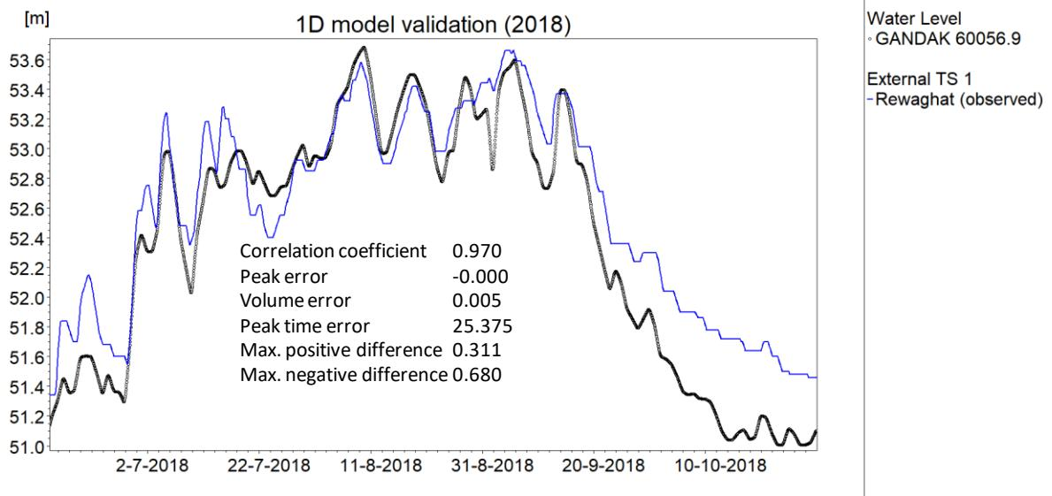
**Figure 5.19: Validation of 1D flow model for 2018 flow data.**
