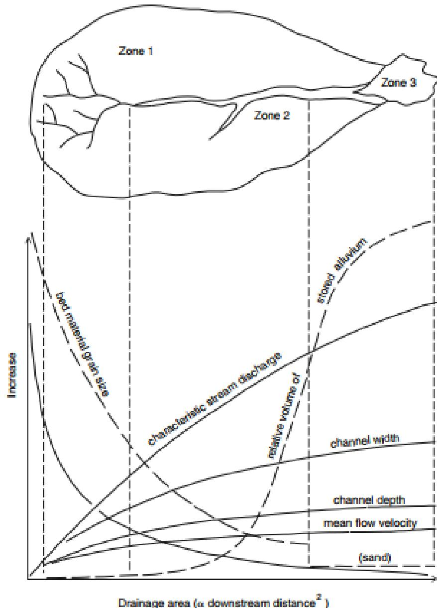
**Figure 4.1: Schematic representation of the variation in channel properties within a drainage basin**
