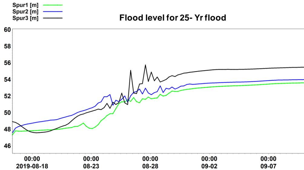
**Figure 5.53: Time series of flood level at three anti-erosion works for 25- yr flood.**
