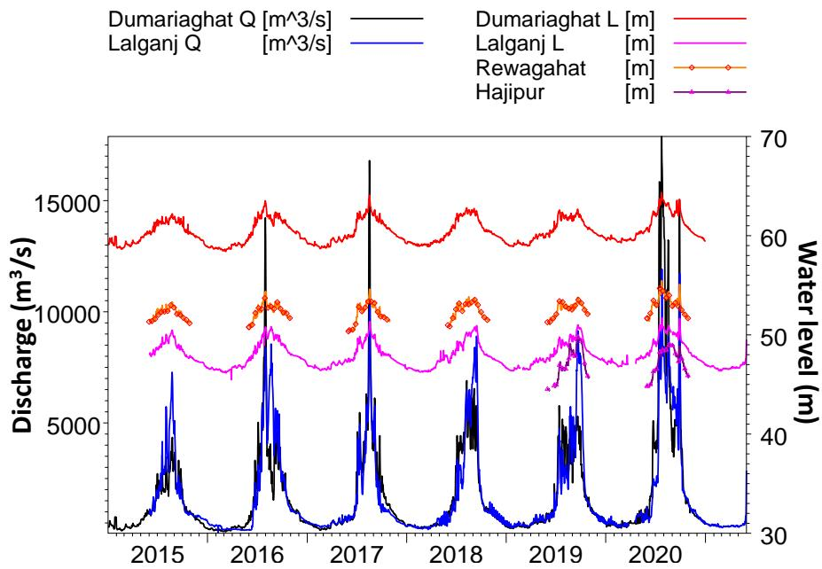
**Figure 3.1: Availability of gauge and discharge data.**
