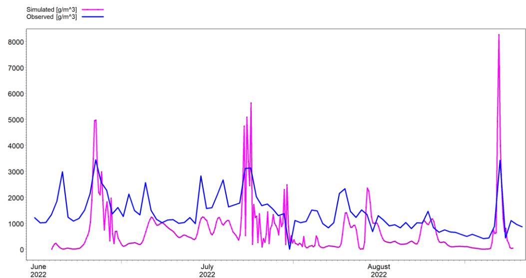
**Figure 5.43: Comparison of simulated and silt load at Baligaon.**
