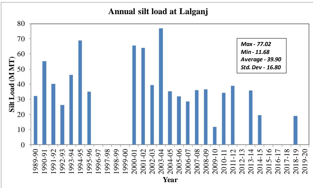
**Figure 3.4: Annual silt load in million metric ton at Lalganj site.**
