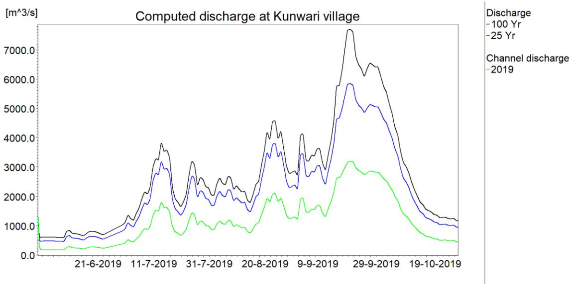
**Figure 5.35: Flood estimates at Kunwari village for various return period computed from MIKE 11 simulation.**
