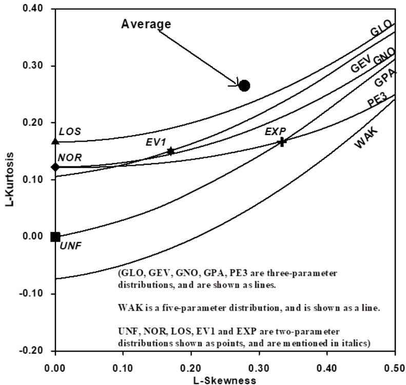
**Figure 5.13: L-moments diagram for annual maximum discharge data for Lalganj GD site.**
