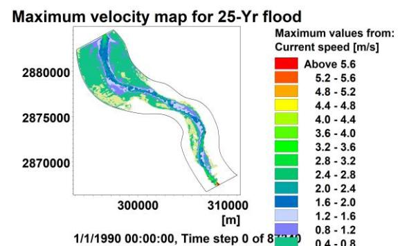
**Figure 5.50: Maximum flow velocity map for 25- Yr flood.**
