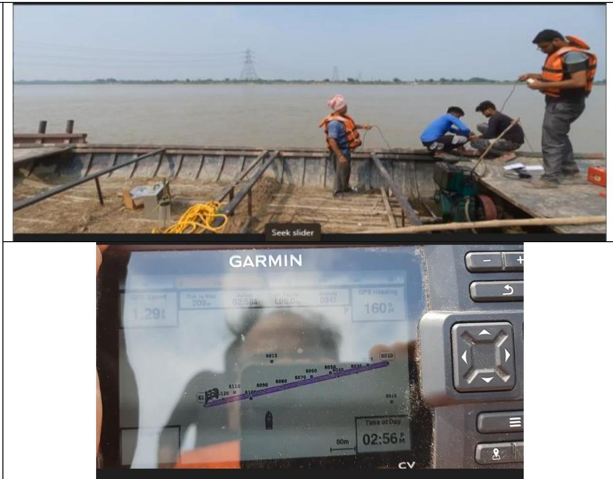
**Figure 3.10: Boat alignment in river using GPS**
