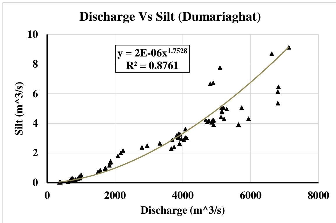
**Figure 5.26: Silt discharge relationship for Dumarighat site based on 2020 observed data.**
