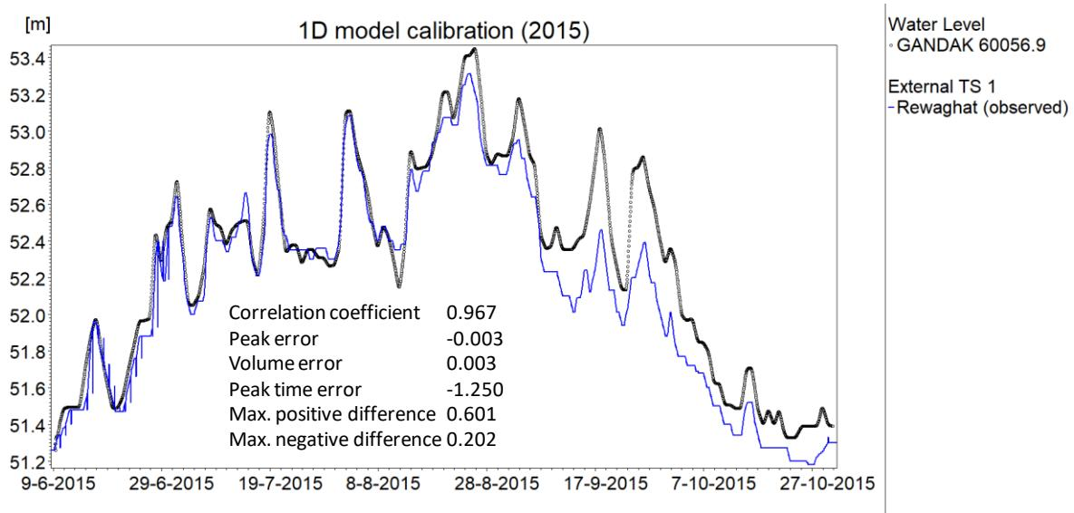
**Figure 5.16: Calibration of 1D flow model for 2015 flow data.**
