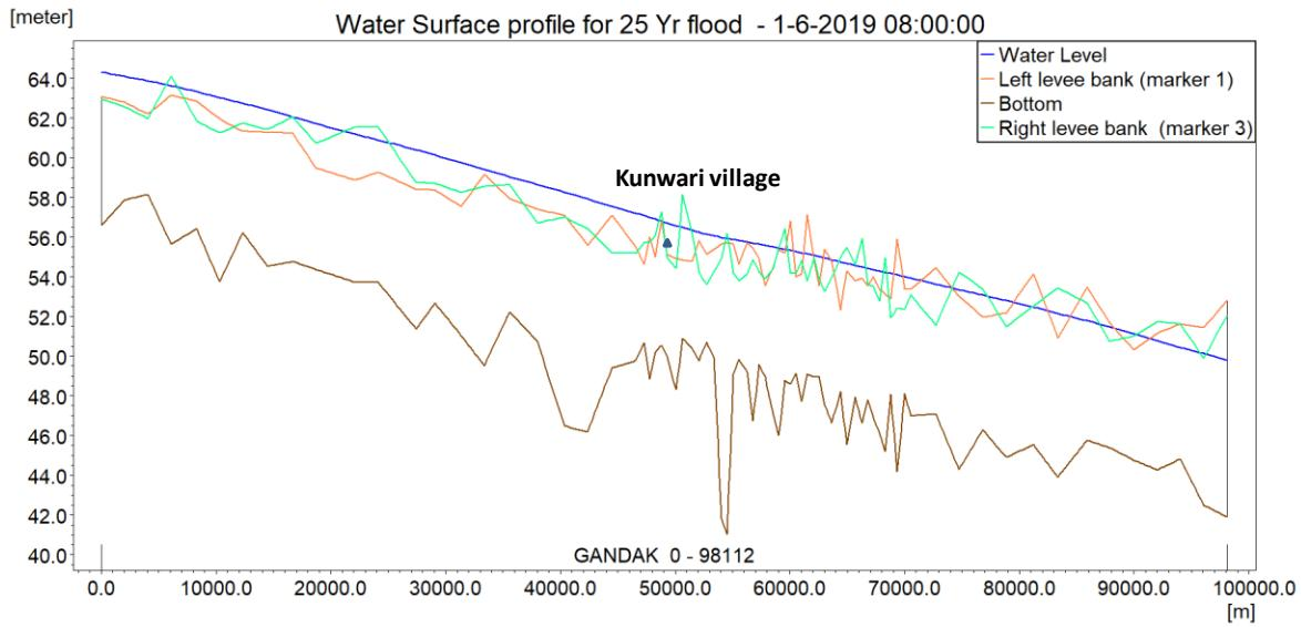
**Figure 5.37: Water Surface profile in Gandak river for 25- Yr flood.**
