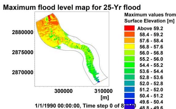
**Figure 5.49: Maximum flood level map for 25- Yr flood.**
