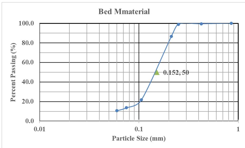
**Figure 3.13: Grainsize distribution chart for bed sediment.**
