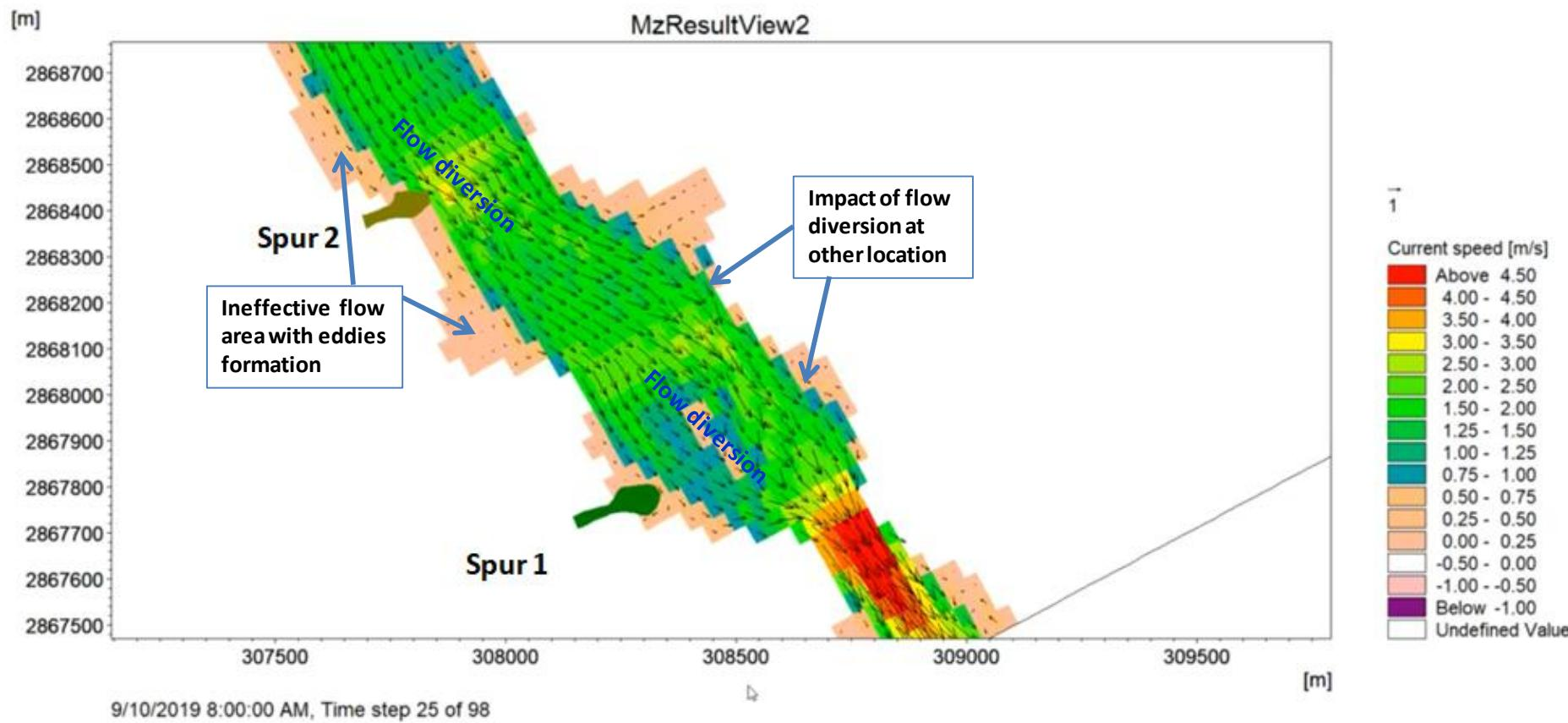
**Figure 5.45: Spatial distribution of flow velocity and flow characteristics.**
