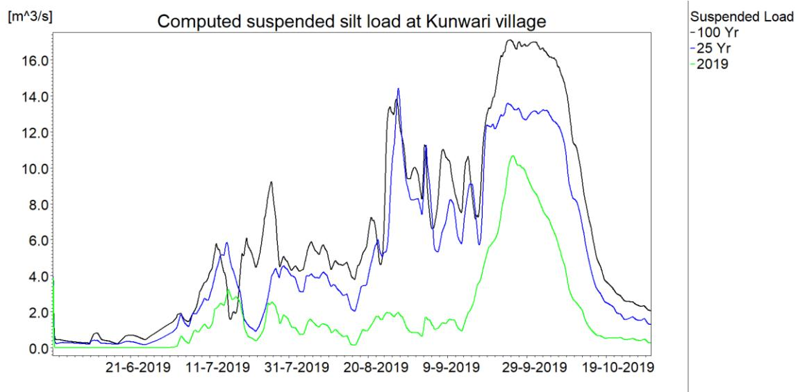
**Figure 5.36: Suspended silt estimates at Kunwari village for various return period computed from MIKE 11 simulation.**
