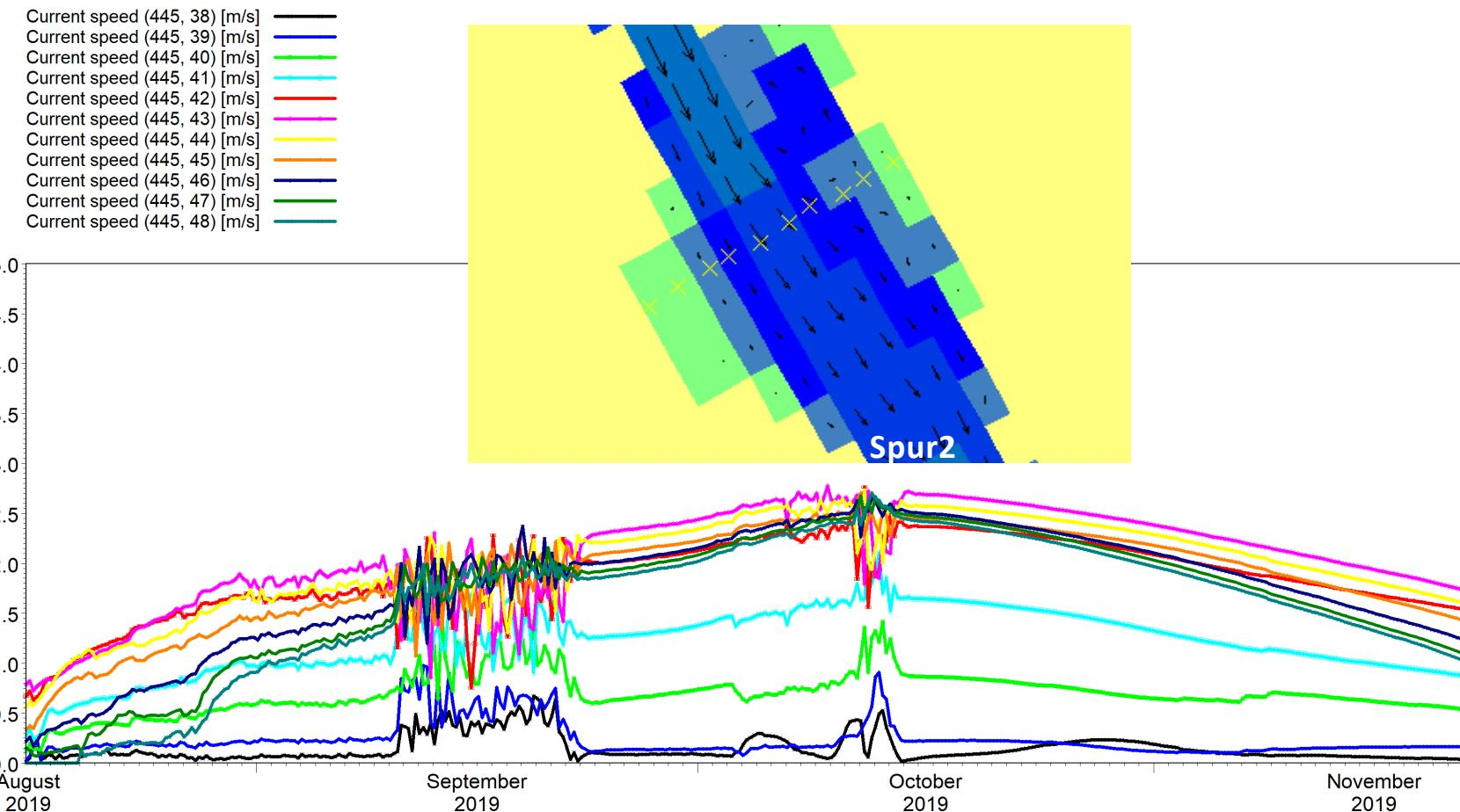
**Figure 5.44: Velocity distribution along the cross section near upstream of 'Spur 2'.**
