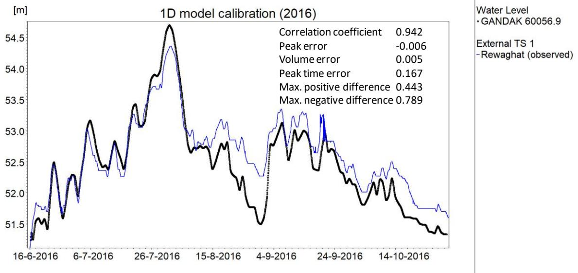
**Figure 5.17: Calibration of 1D flow model for 2016 flow data.**
