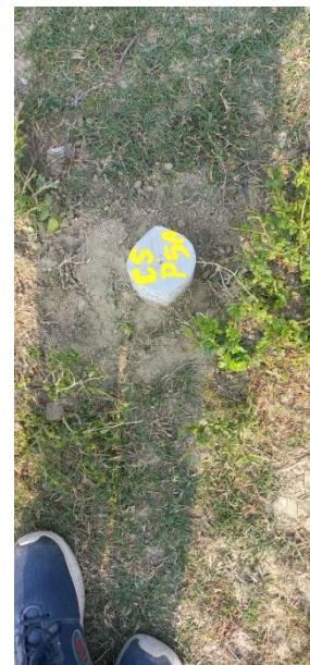
**Pillar (TBM) at cross section locations**
