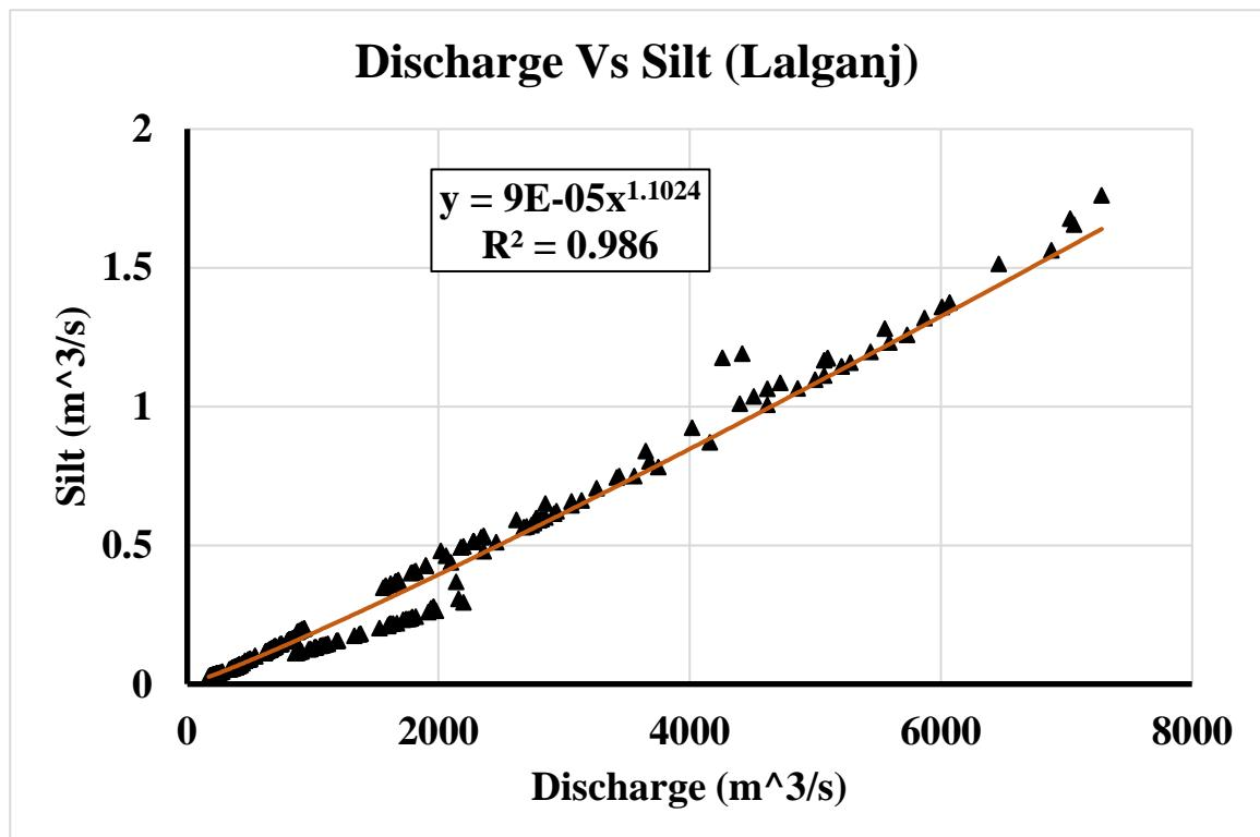
**Figure 5.27: Silt discharge relationship for Lalganj site based on 2019 observed data.**
