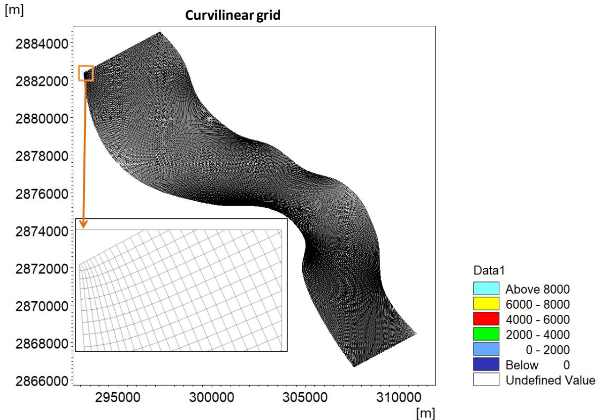
**Figure 5.31: Curvilinear grid generated for the study reach.**
