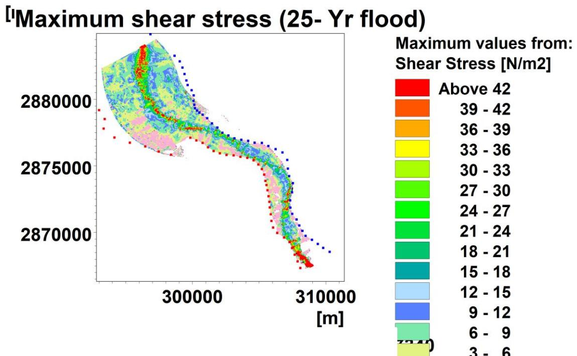
**Figure 5.58: Maximum shear stress map for 25- yr flood.**
