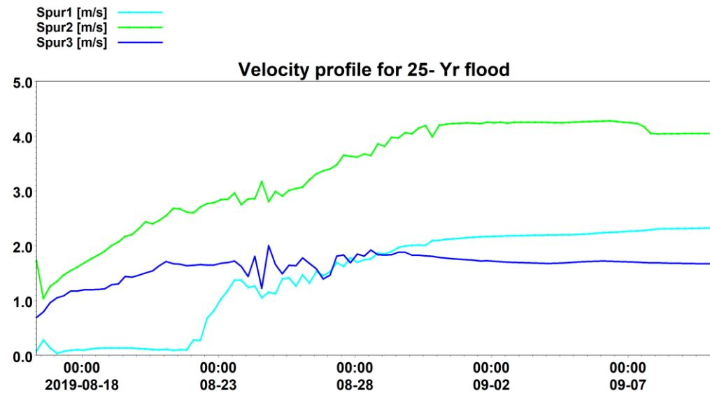
**Figure 5.54: Time series of flow velocity at three anti-erosion works for 25- yr flood.**
