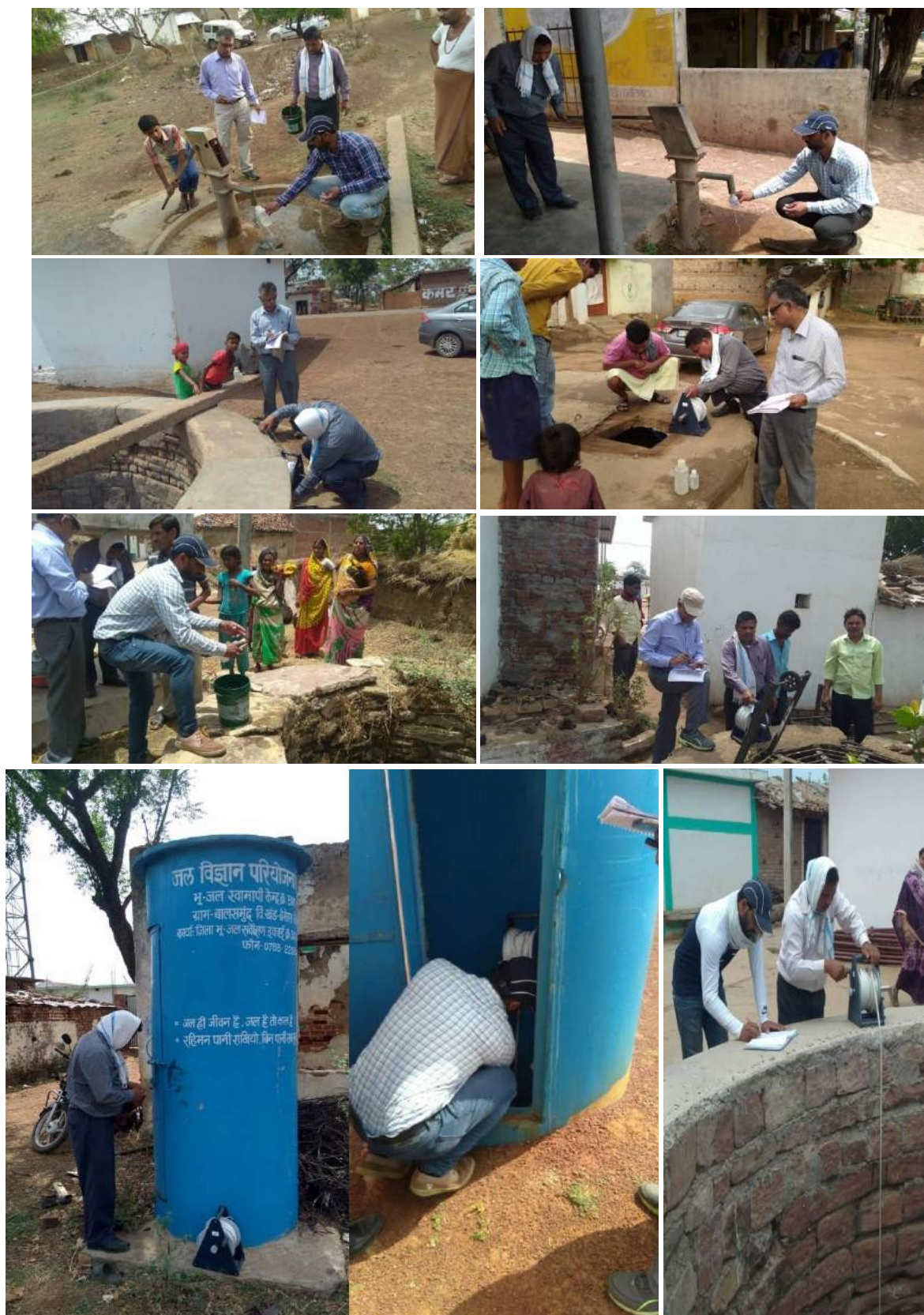
Fig. 2(c). Photographs showing groundwater sampling from handpumps, open wells, piezometric wells and groundwater level measurement in the study area
