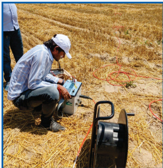
Geophysical survey using Electrical Resistivity Tomography (ERT) in IGNP, Rajasthan
