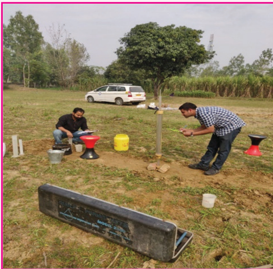
Infiltration and hydraulic conductivity tests in the catchment of Sot river
