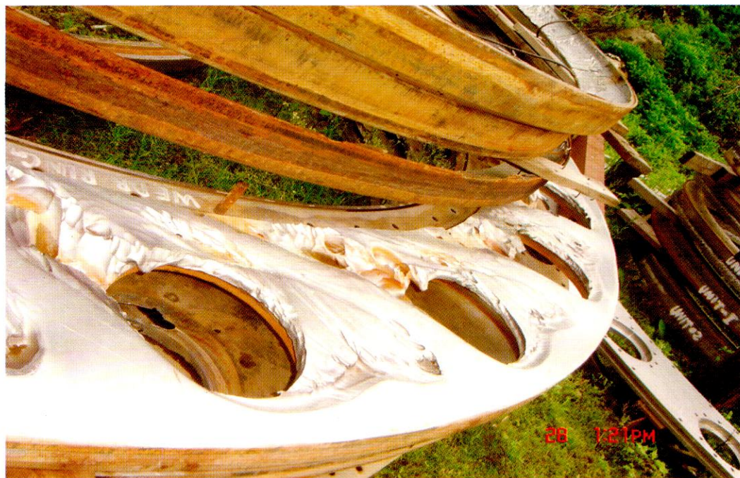
Fig. 4.5 Damage of turbine blade due to fine sediment in Nathpa-Jhakri hydro power project
