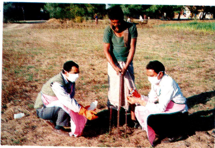
Radiotracer injection for estimation groundwater recharge due to rainfall / irrigation. Popularly termed as tritium tagging technique.
