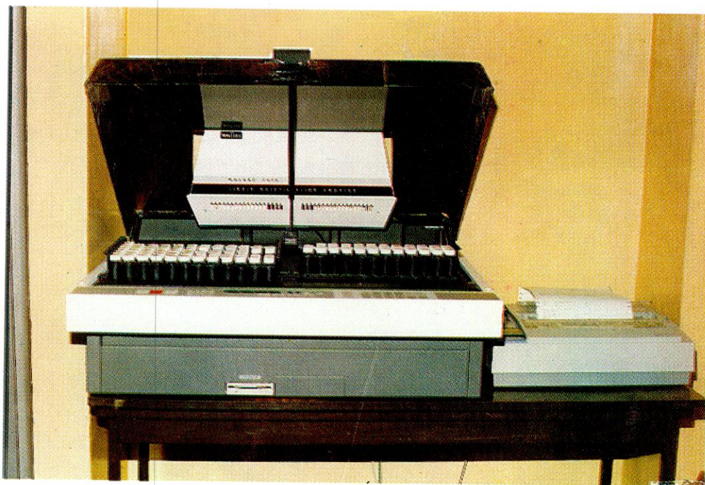
Normal liquid scintillation spectrometer for measuring \alpha and \beta artificial radioisotopes
