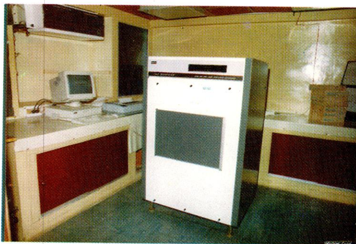
Ultra low-level liquid scintillation spectrometer for measuring very low-level activity of \alpha & \beta radioisotopes including environmental tritium & carbon-14
