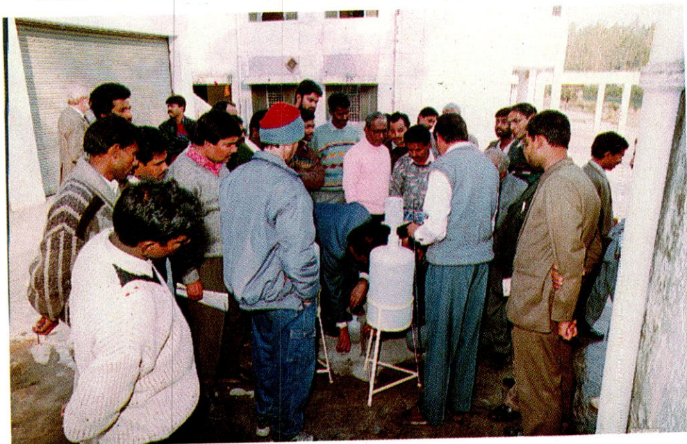
Sampling of groundwater for age determination using Carbon-14 dating technique
