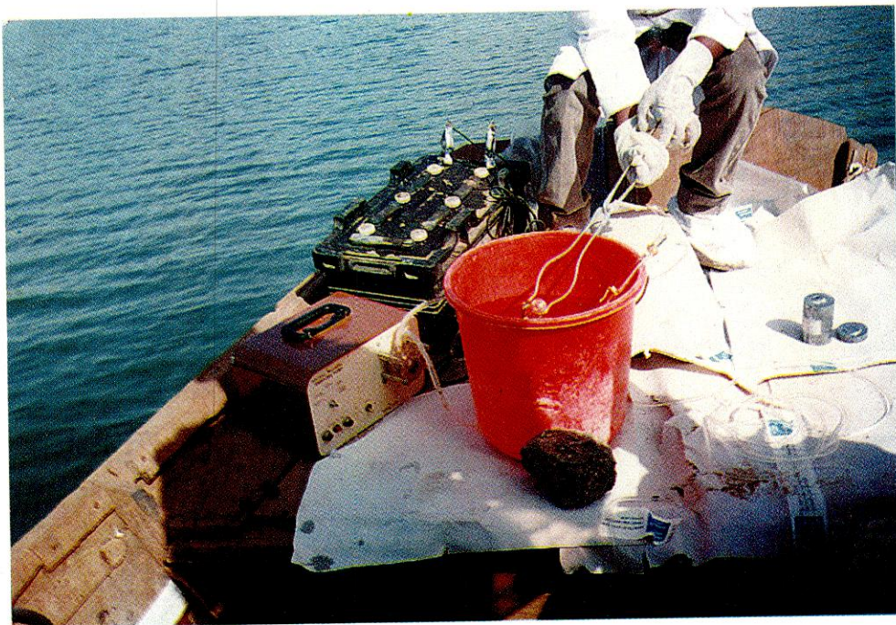
Preparing radiotracer sample for injecting it into a reservoir to detect the leakage points in the reservoir
