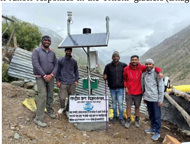
Installed AWS at the Yotche site, Triloki glacier site, Bhaga basin, Keylong, HP.
