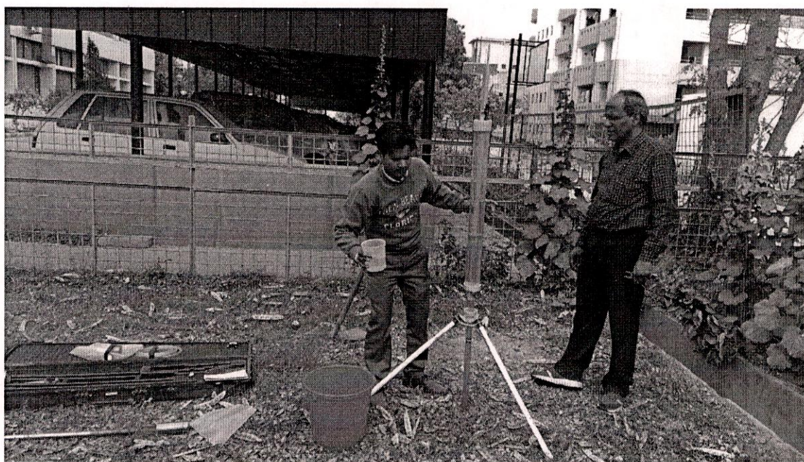
Fig 6.2: Field saturated hydraulic conductivity using Guelph Permeameter.
