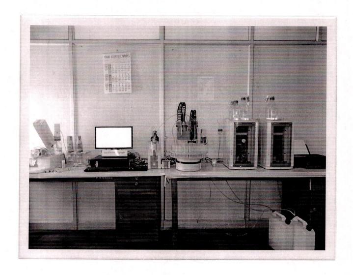
First of all the sample is introduced then flows through the guard and into the analytical ion exchange columns where the ion exchange occurs . After separation, the suppressor reduces the conductivity of the eluent and increase the conductivity of the analytes . So they are delivered to the detector . A computer and software are used to control the system .
