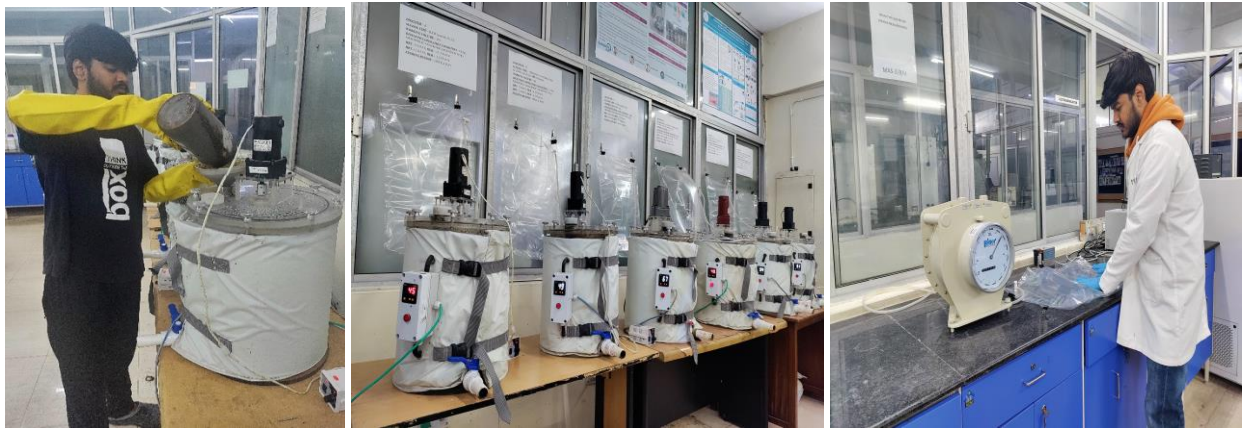
Fig.6. a) Feeding on digesters b) Digesters under operation at varying HRTs c) Biogas composition measurement
