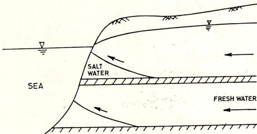
FIG.1: IDEALISED CROSS-SECTION OF A TWO LAYER COASTAL AQUIFER SYSTEM
