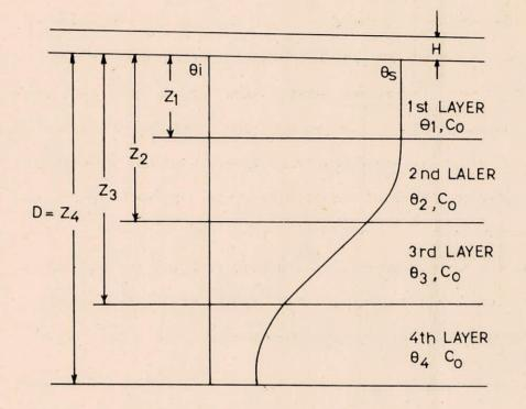
Fig. 1 : Variation of soil moisture with respect to depth for a typical soil
