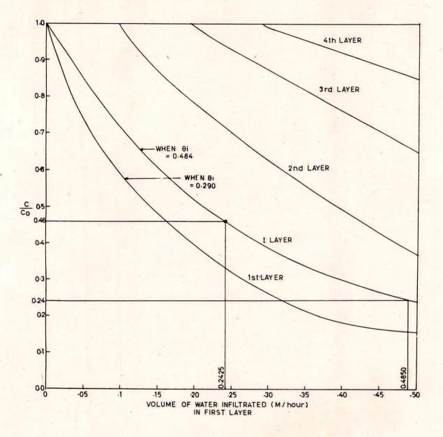
Fig. 6 : Breakthrough curve as a function of relative salt concentration and volume of infiltrated water in different reservoirs
