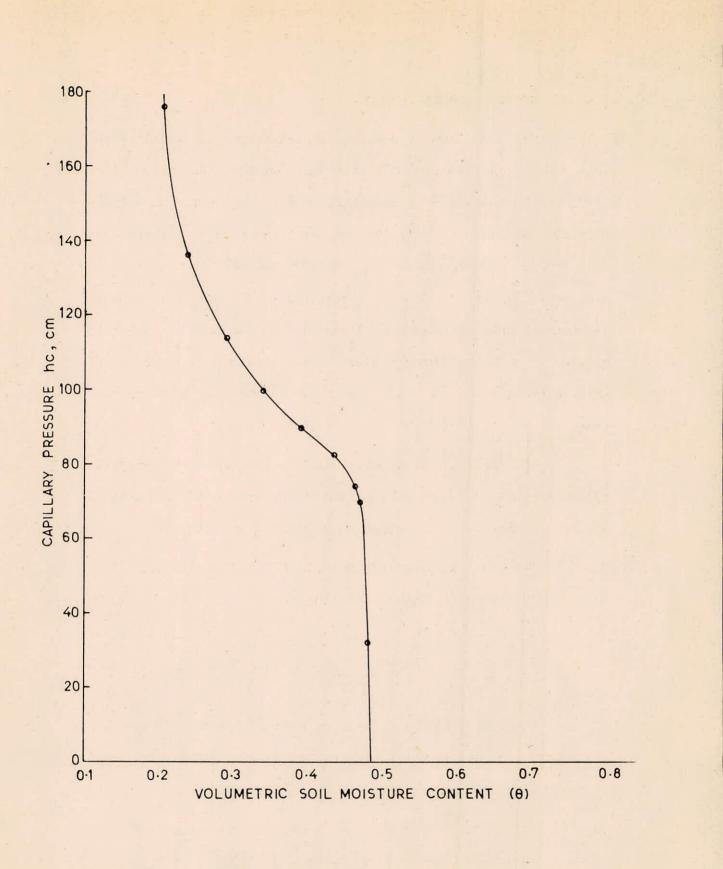
Fig. 2 : Variation of capillary pressure (hc) with volumetric soil moisture content ( $\Theta$ ) for touchet silt loam
