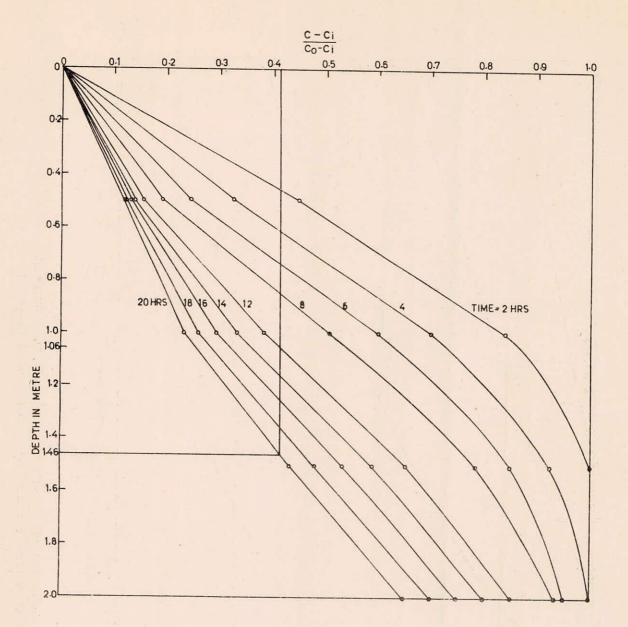
Fig. 5 : Variation of non-dimensional salt concentration with depth for different time periods
