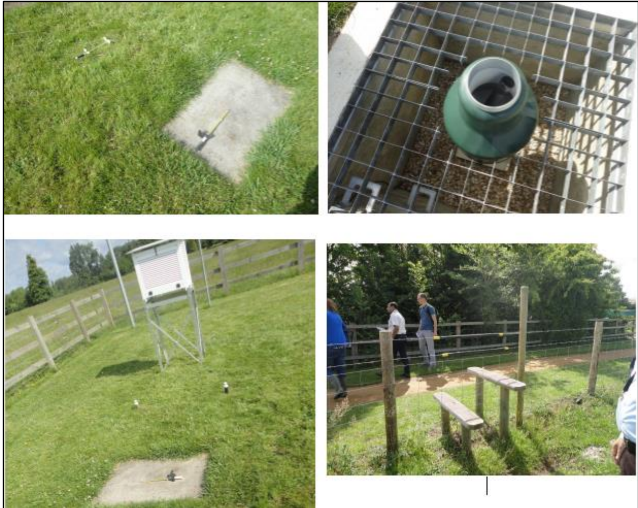
Meteorological site showing the Weighing type rain gauge at CEH, Wallingford
