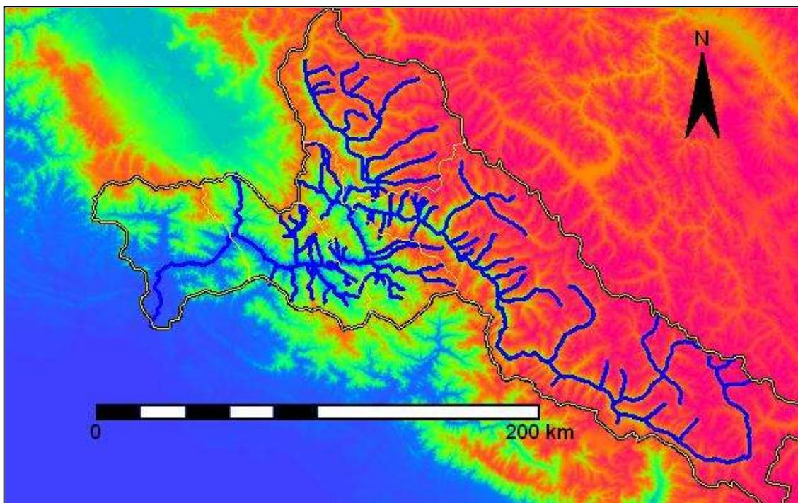
**Figure – 2.2:** Layout of Chenab basin boundary over the DEM
