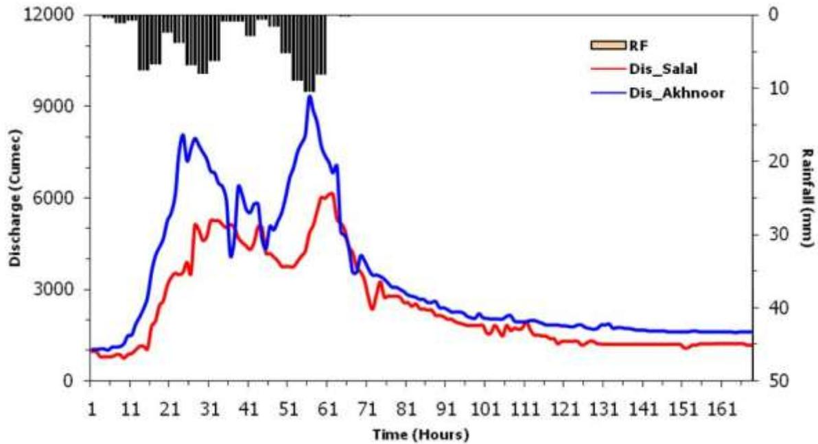
**Figure – 2.11:** Observed flow at Salal & Akhnoor and average basin rainfall pattern (3-hourly) during September 1 – 6, 2006
