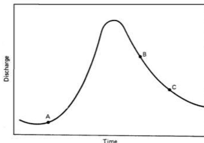
**Figure – 4.1:** A discharge hydrograph
