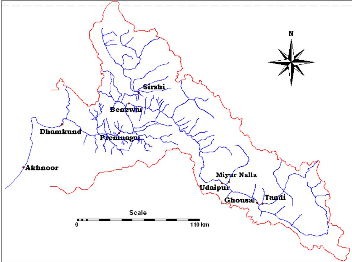
**Figure – 2.5:** Network of river gauging stations in Chenab basin up to Akhnoor
