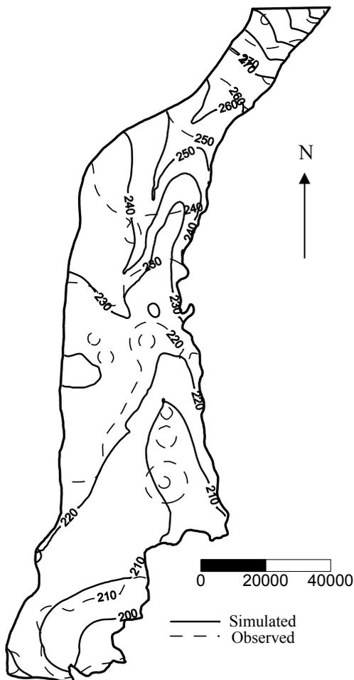
Fig. 3 Simulated and observed heads for Aquifer I for steady state.
