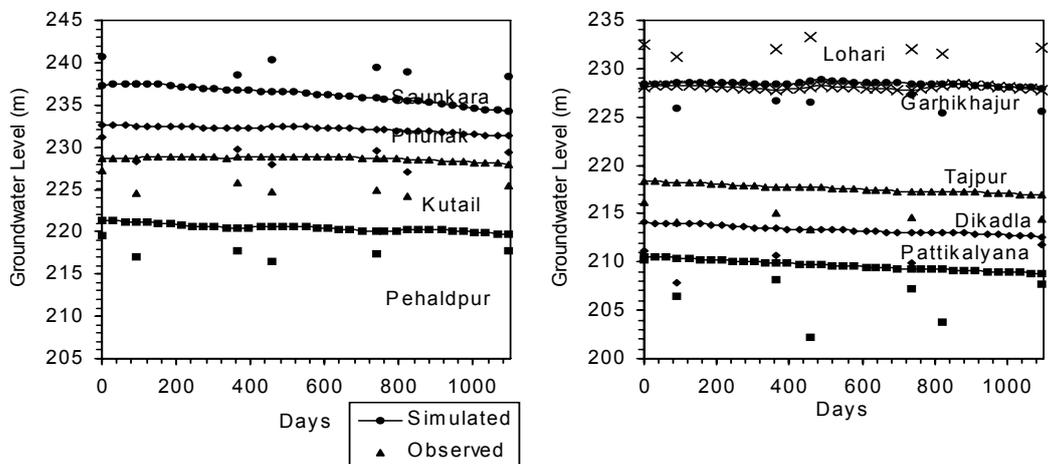
Fig. 5 Observed and simulated groundwater level hydrographs for Aquifer II.
