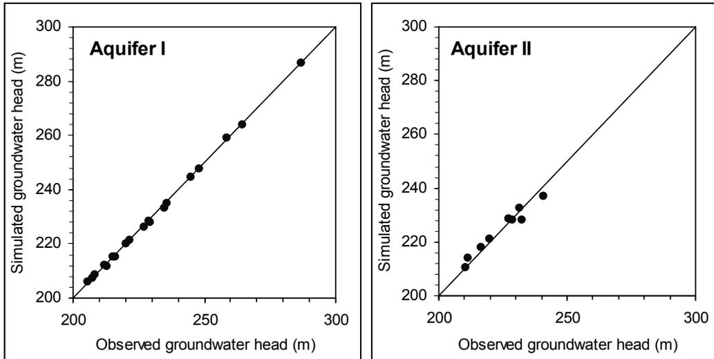
Fig. 2 Scatter plot of simulated and observed groundwater levels for steady state.
