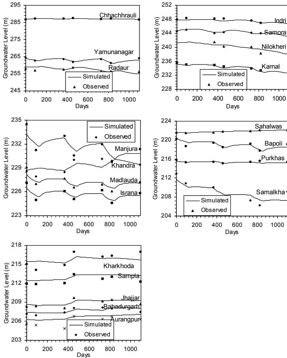
Fig. 4 Observed and simulated groundwater level hydrographs for Aquifer I.
