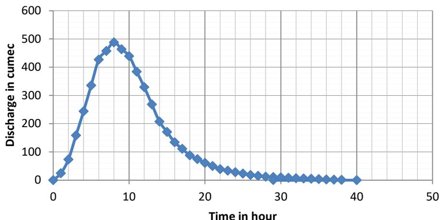
Figure 4. Ordinates of 1-hr SCS Unit Hydrograph in Cumecs
