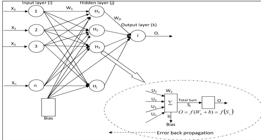
**Fig.1:** An artificial neuron showing its function
