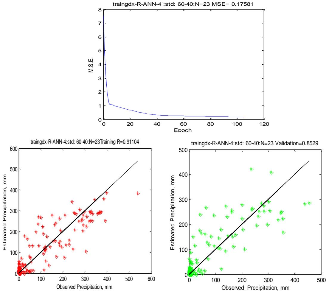
**Fig. 2** Performance of “traingdx” training algorithm with 23 neurons with 60% length of data set used for training and the rest of that used for validation ANN modeling (precipitation).
