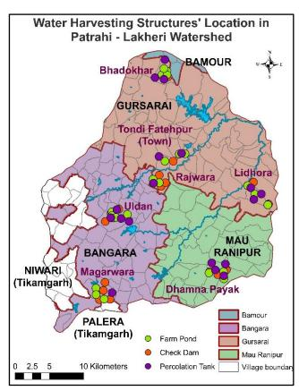
suitable location to supplement irrigation. The plan provides suitable locations and component under which it can be constructed. (see Table 3). Apart from this, for domestic usage like drinking, bathing and cooking, rooftop rainwater harvesting can be an effective solution to store water.
