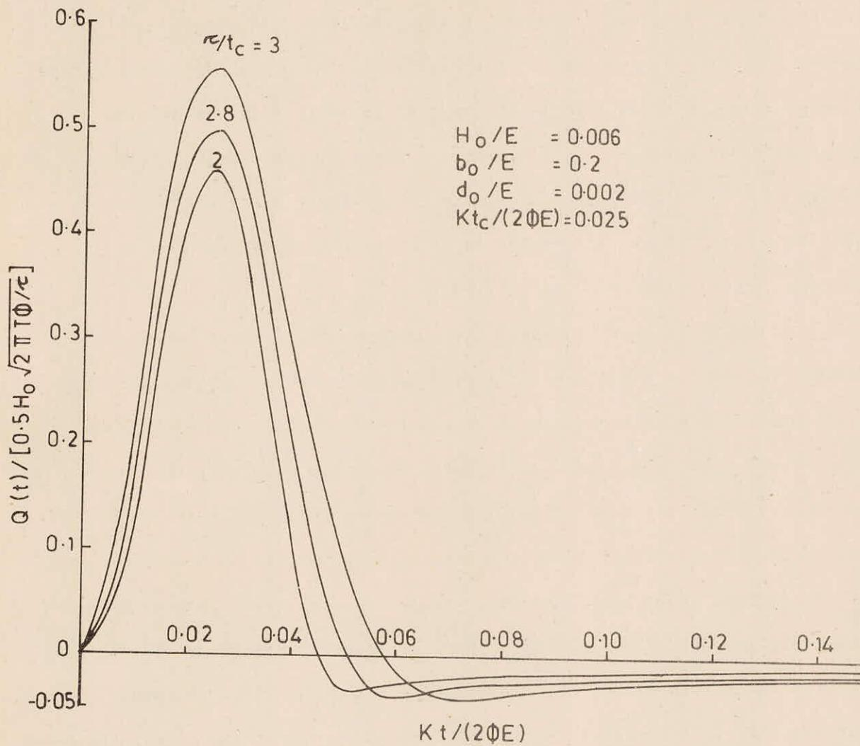
Fig.2(c) Exchange of flow between a river and an aquifer during the passage of a flood for different durations, the flood peak occurs at  $Kt / (2\Phi E) = 0.025$ , and initial width of the river,  $b_0 / E = 0.2$
