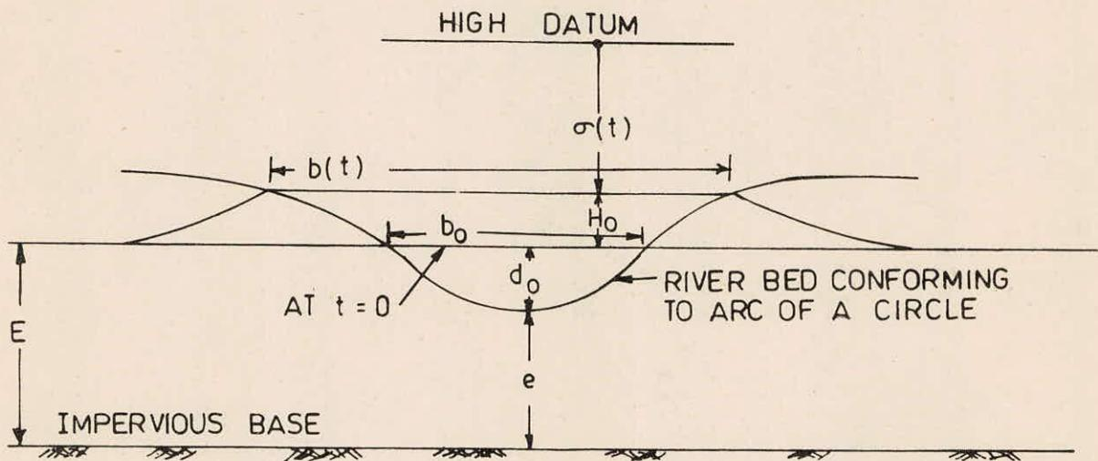
Fig.1(a) Schematic section of a river whose width changes gradually during the passage of a flood
