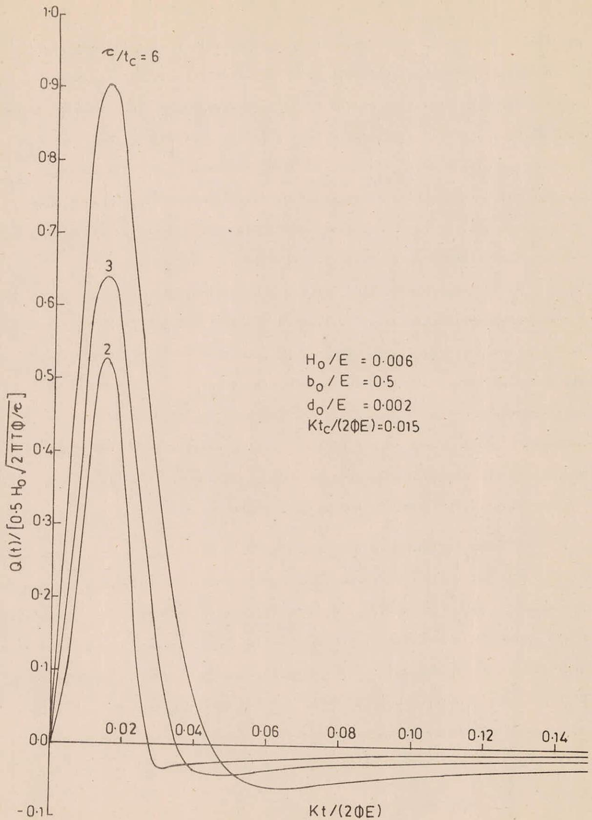
Fig. 2(b) Exchange of flow between a river and an aquifer during passage of a flood for different durations, the flood peak occurs at  $Kt/(2\phi E) = 0.015$  initial width of the river,  $b_0/E = 0.5$
