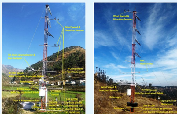
Fig. 1. The Automatic Weather Station (AWS) installed at Henval watershed near Nagini Village and Kanataal Village, TehriGarhwal (Uttarakhand)
