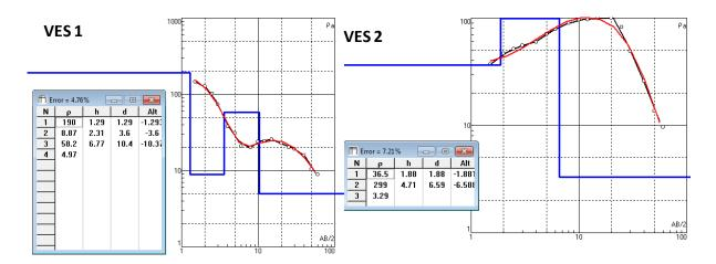
Fig. 2. Resistivity survey results for the Agra site
