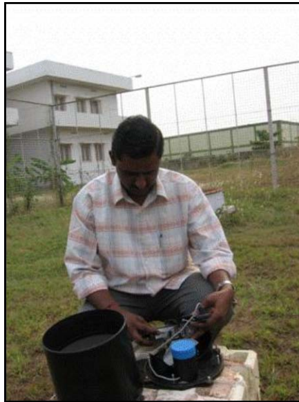
Fig. 23. Down loading data through shuttle from Digital rain gauge
