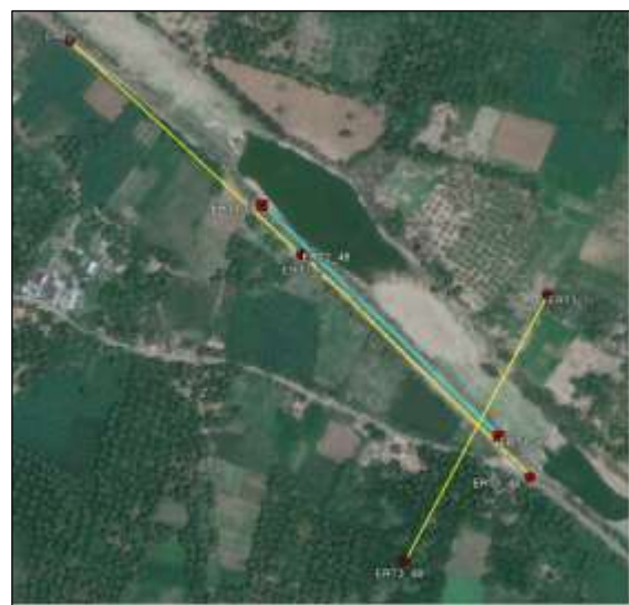
Figure 30: Location for the Electrical Resistivity Tomographic survey near Vommavaram village alignment in the vicinity of the Varaha River.
