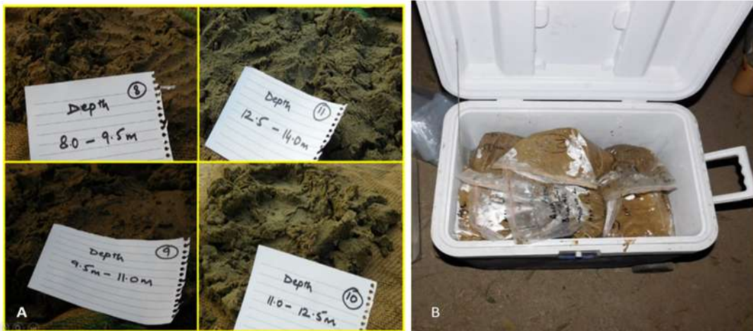
Figure 19: Soil samples collected from exploratory bore of Agra site at various depths.
